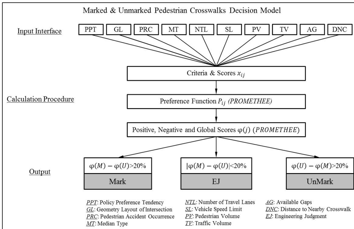
Figure 9 Flow Chart of Developed Mark/Unmark Choice Tool
