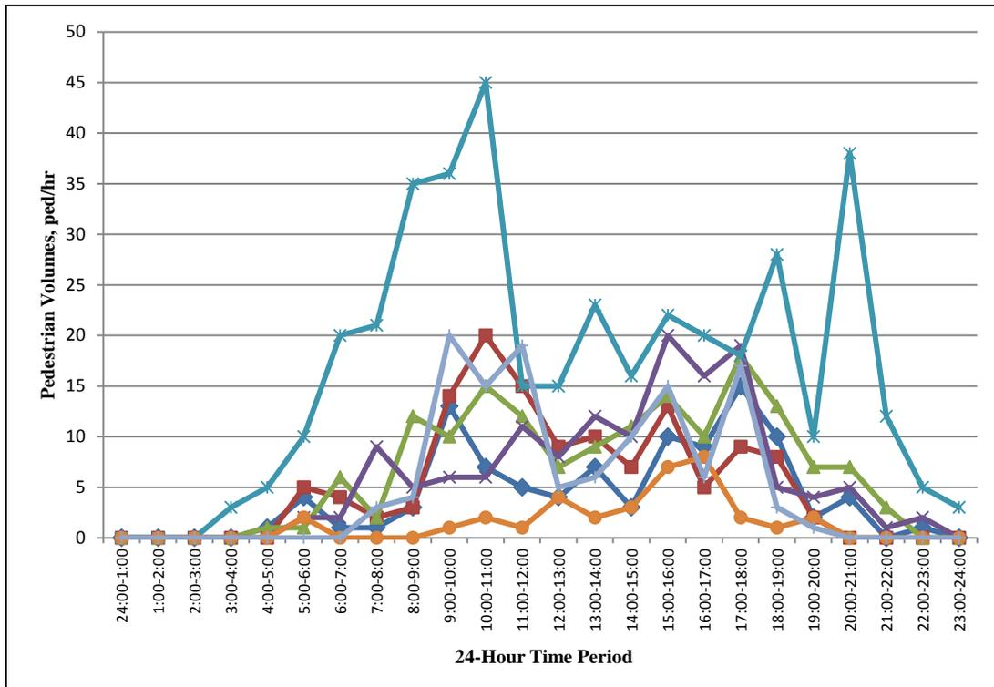
Figure 8 Pedestrian ADTs at Selected Signalized Intersections
