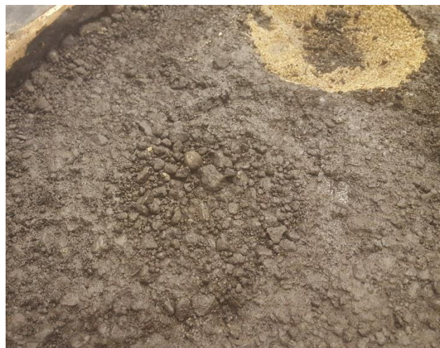
Figure 11. Washed fines after performing the permeability test.
