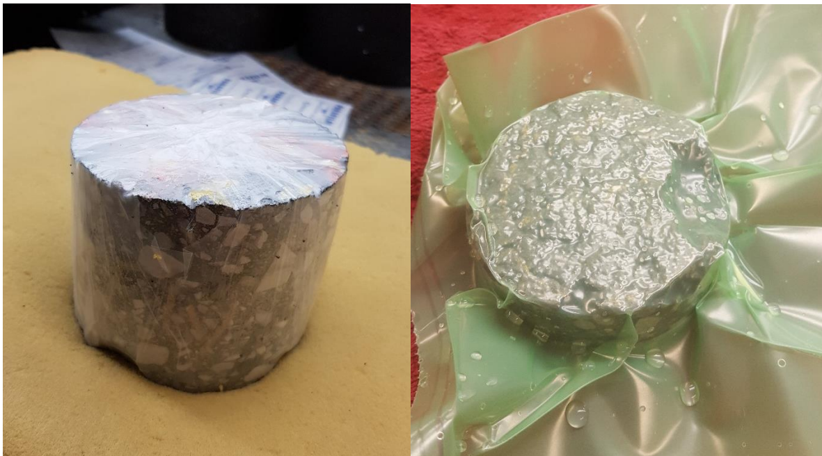
Figure 13. Test methods for bulk specific gravity of cores: left – Parafilm, right – Corelok.
