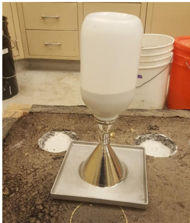
Figure 5. Sand cone apparatus on the CIR mat.
