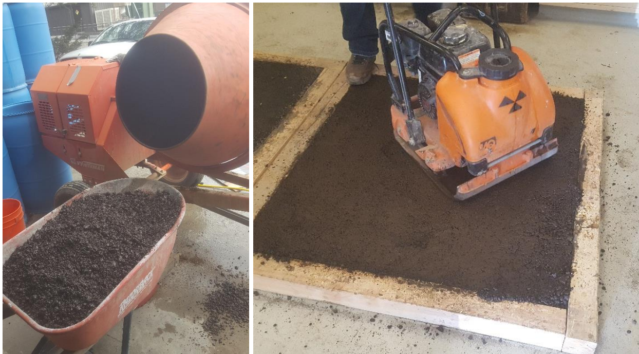
Figure 8. Laboratory CIR mixture production and compaction using concrete mixer and vibratory plate compactor.
