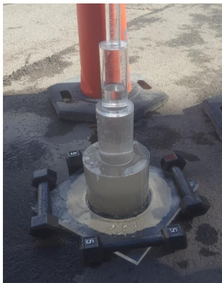
Figure 7. NCAT Field Permeameter apparatus on the CIR mat.
