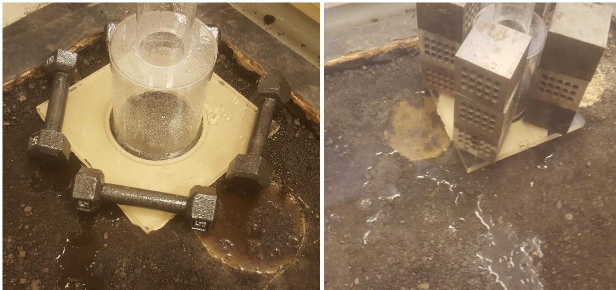
Figure 10. Water leaks during the permeability test.
