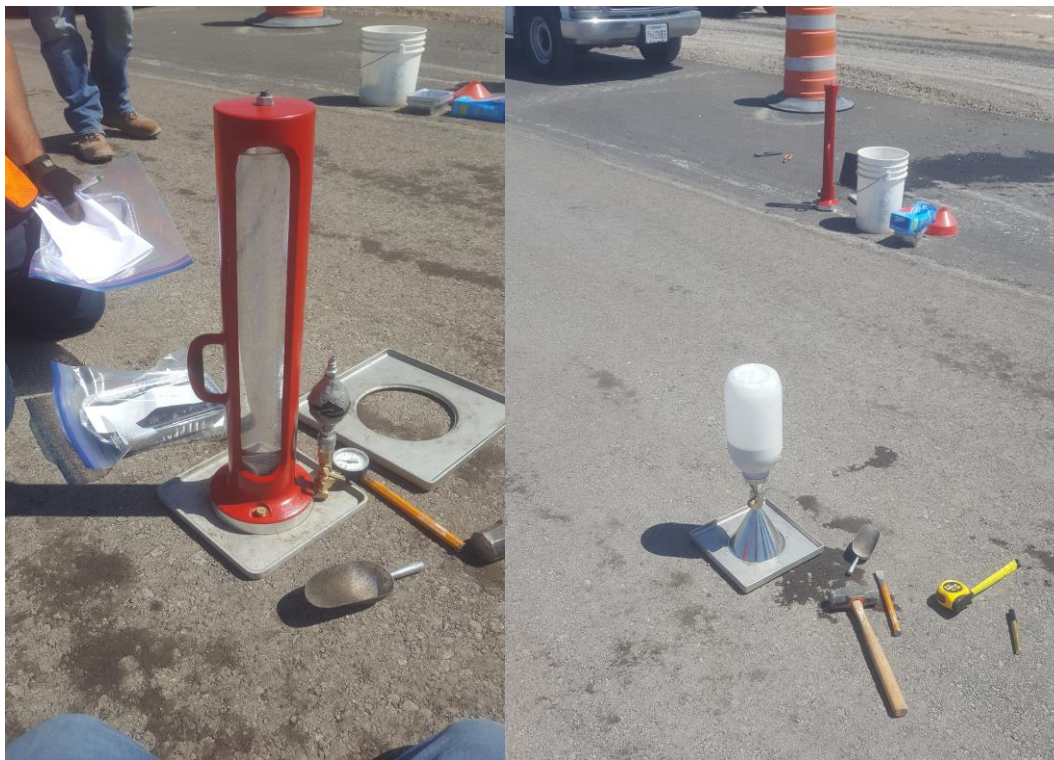
Figure 29. In-place density on the Fernley CIR project: rubber balloon and sand cone.
