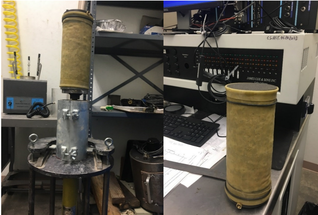
Figure 4.11. Compacted sample with membrane, porous stones and O-rings.
