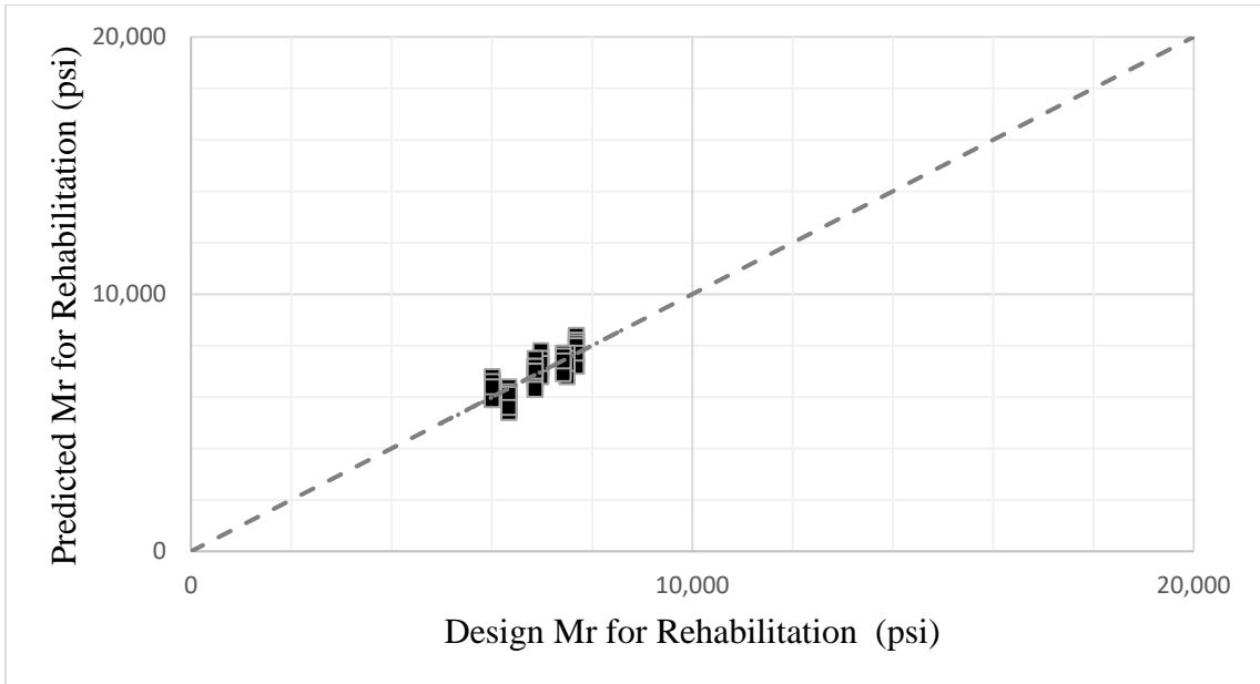
Figure 7.5. Variation of design resilient modulus versus predicted resilient modulus of subgrade (using UCS) for rehabilitation design.
