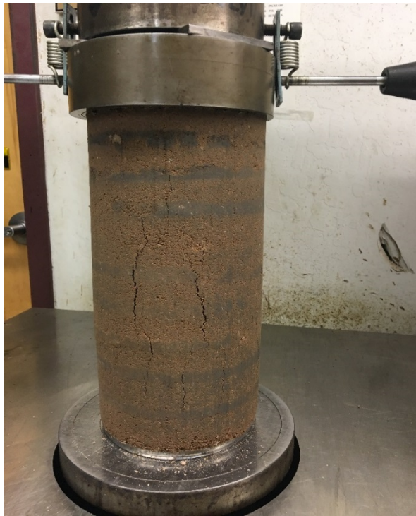
Figure 4.22. Sample after the UCS test.
