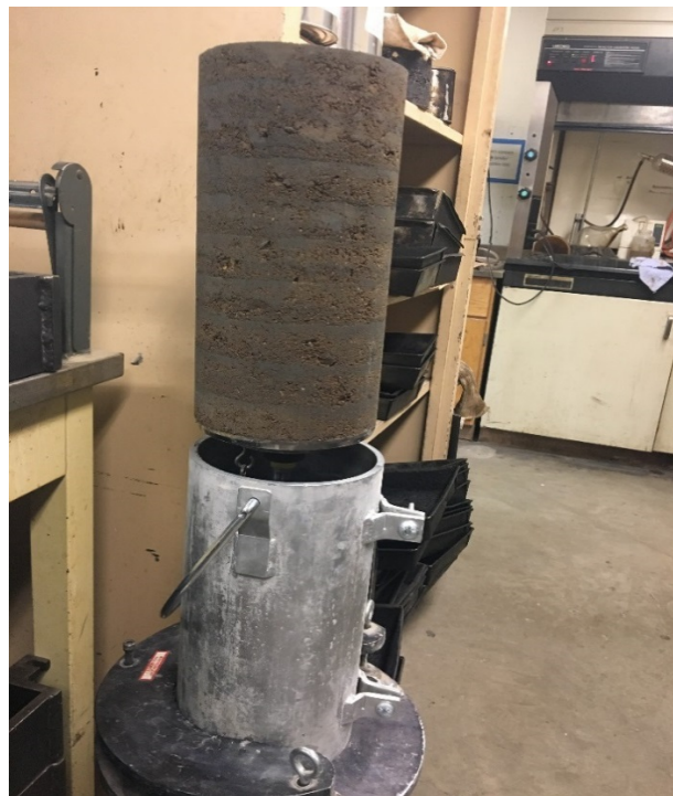
Figure 4.21. Extruded UCS sample.
