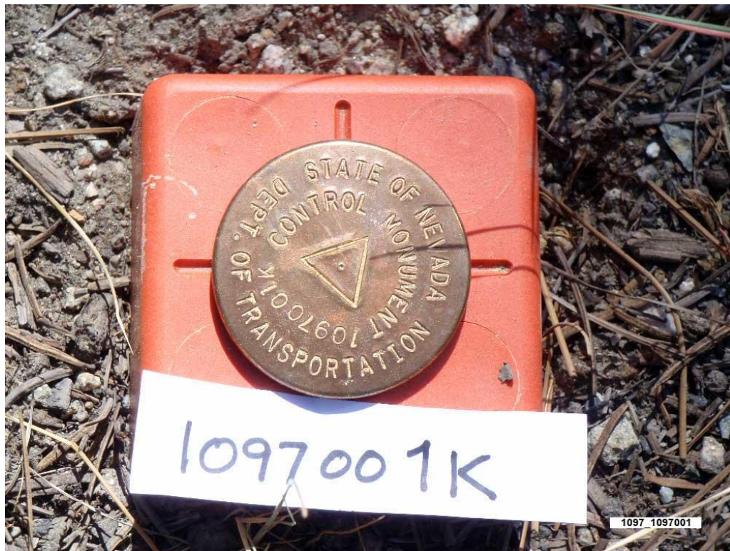
K-Construction Control Point / No Spirit Level Elevations
