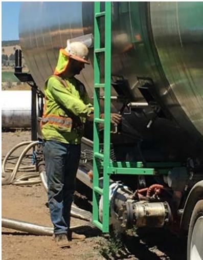
**Figure 4.7. Photo. Sampling of asphalt binders.**
