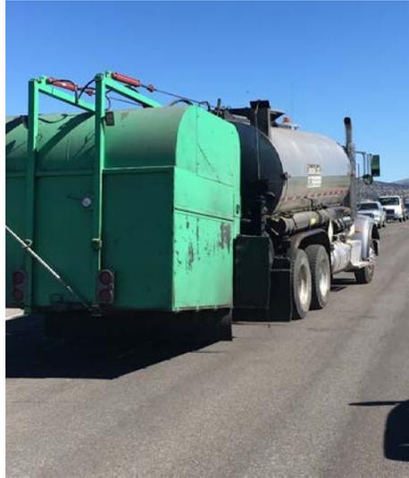
**Figure 4.2. Photo. Asphalt binder distributor with emissions capture apparatus.**
