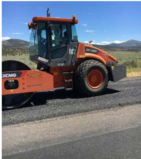
**Figure 4.3. Photo. Single-drum steel roller.**
