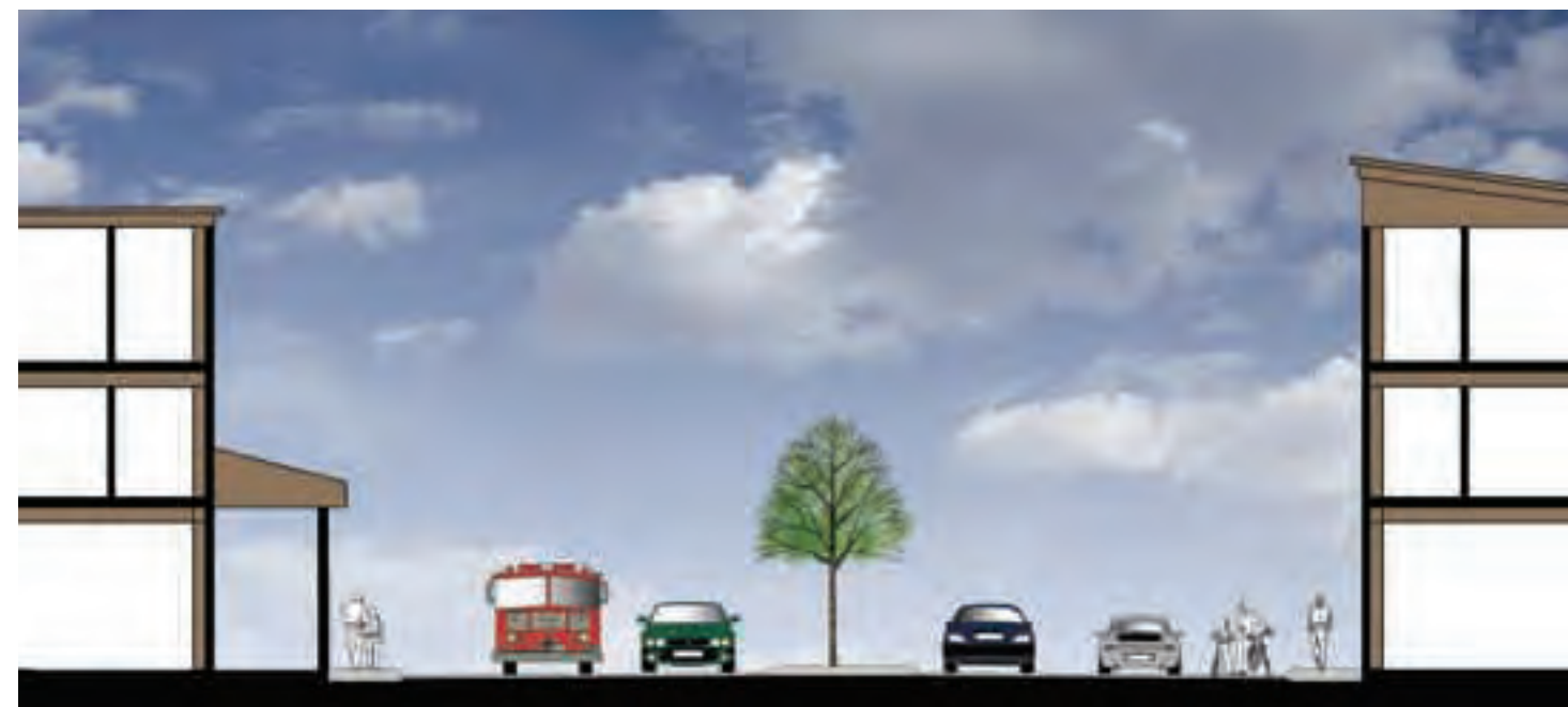
(4) An 80' right-of-way accommodates dual travel lanes and a planted median. A striped bike lane accommodates cyclists through the community center. Pedestrian amenities may be enhanced with widened sidewalks.
