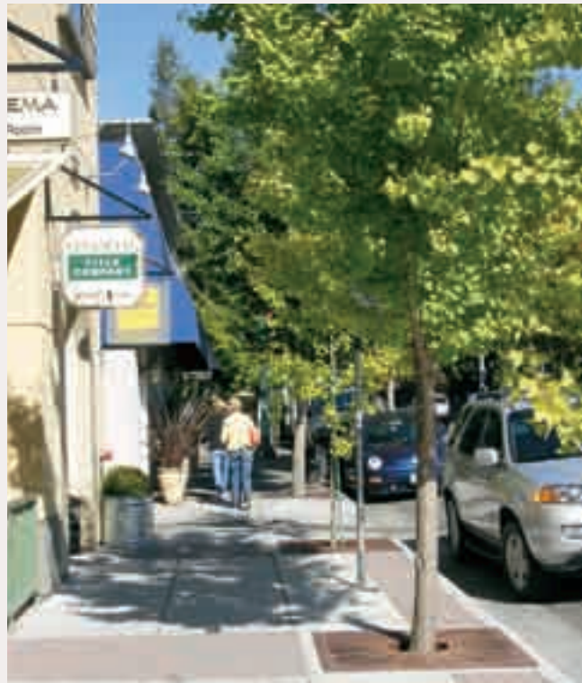
(1) The primary design objective for community interface zones is the highway's ability to accommodate a variety of town-center activities without reducing its function as a through street. On-street parking buffers pedestrians from travel lanes and helps slow traffic through town.
