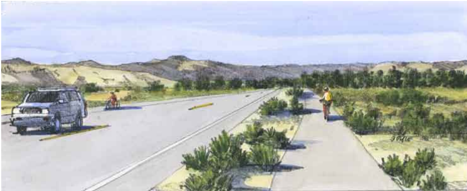
(1) Road shoulders can be improved for truck safety while preserving existing vegetation and incorporating a designated bike lane.
