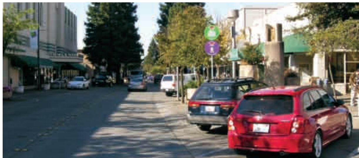
(7) Where rural highways go through towns, traffic calming features such as bulb-outs at crosswalks and angled parking combined with street furnishings create a more pedestrian friendly environment.
