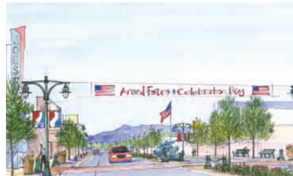
(4) Creating a street system and aesthetics that support the community vision can be achieved through the incorporation of transportation art, pedestrian lighting, bollards, and pedestrian amenities. Planted medians and accentuated paving at pedestrian crossings bring the scale of the highway into alignment with the surrounding development.
