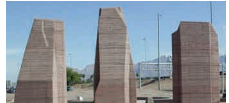
(6) Contemporary materials suited to the region, such as the rammed earth sculpture shown above, provide excellent alternatives to traditional materials that may be expensive, hard to maintain, or not durable.
