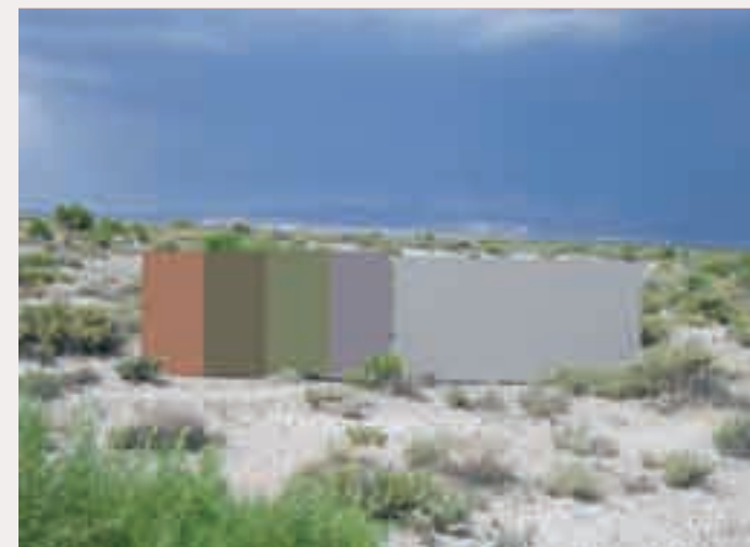
(3) The color palette was field tested in morning, afternoon and evening conditions.
