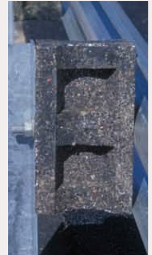
(3) Materials like this recycled plastic modular unit can be used in roadway construction.
