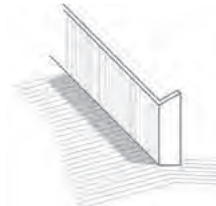
(4) A wall return of three feet is recommended for noise walls outside the clear zone at the beginning of the wall facing the driver.
