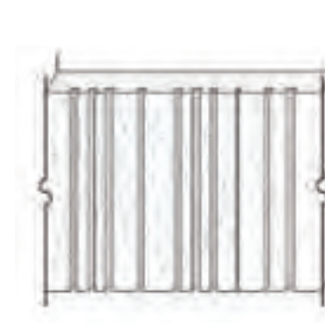
(3) Preferred prototypical surface pattern is rusticated variable vertical ribbing. Dimensions vary between 2"-8" apart.
