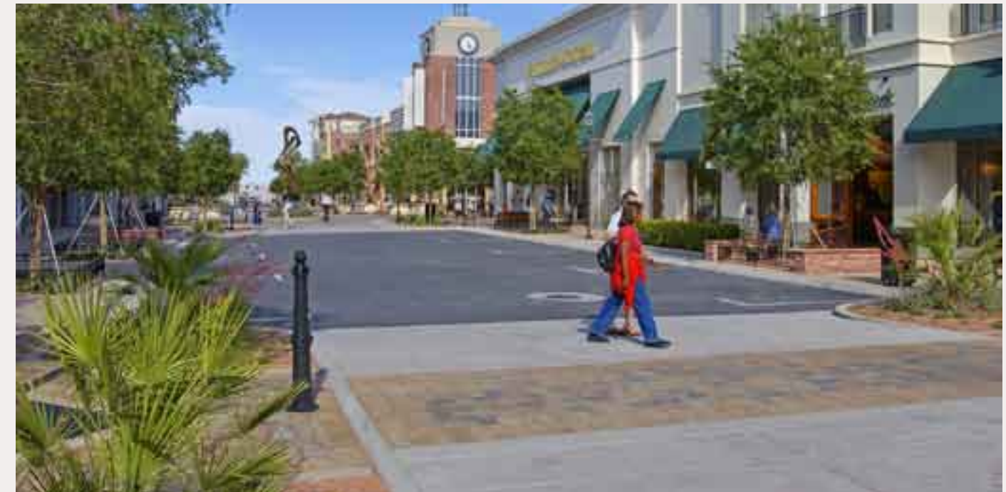
(3) Use of colored paving differentiates pedestrian crossings and elevates the pedestrians importance.
