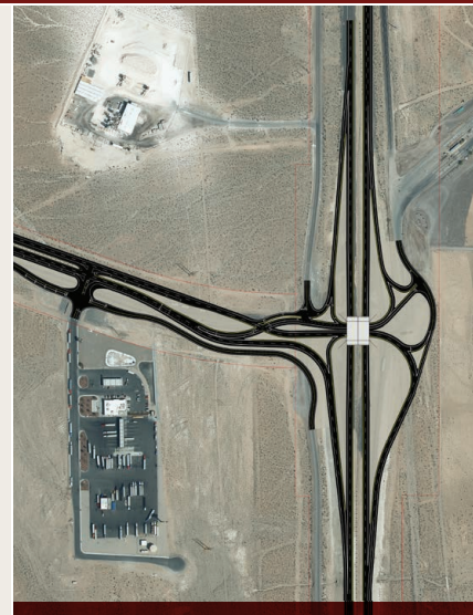
Modified diverging diamond interchange concept
