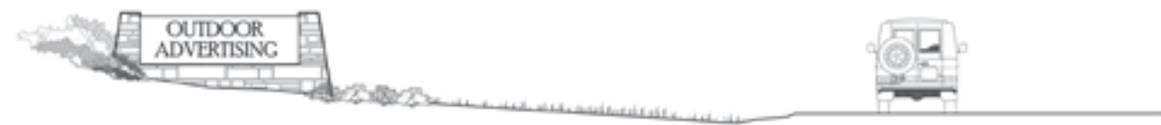
(2) Outdoor advertising can be framed by natural materials and landscaping and built into the ground in order to limit scenic distractions.
