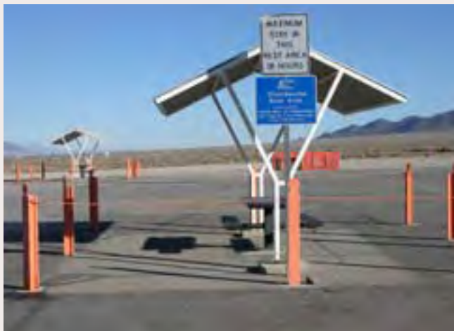
(2) Rest areas typically contain large amounts of paving and distracting barriers that decrease their aesthetic appeal and ability to provide an inviting place for motorists to stop. Corridor Plan guidelines suggest modifications to enhance function and appearance.
