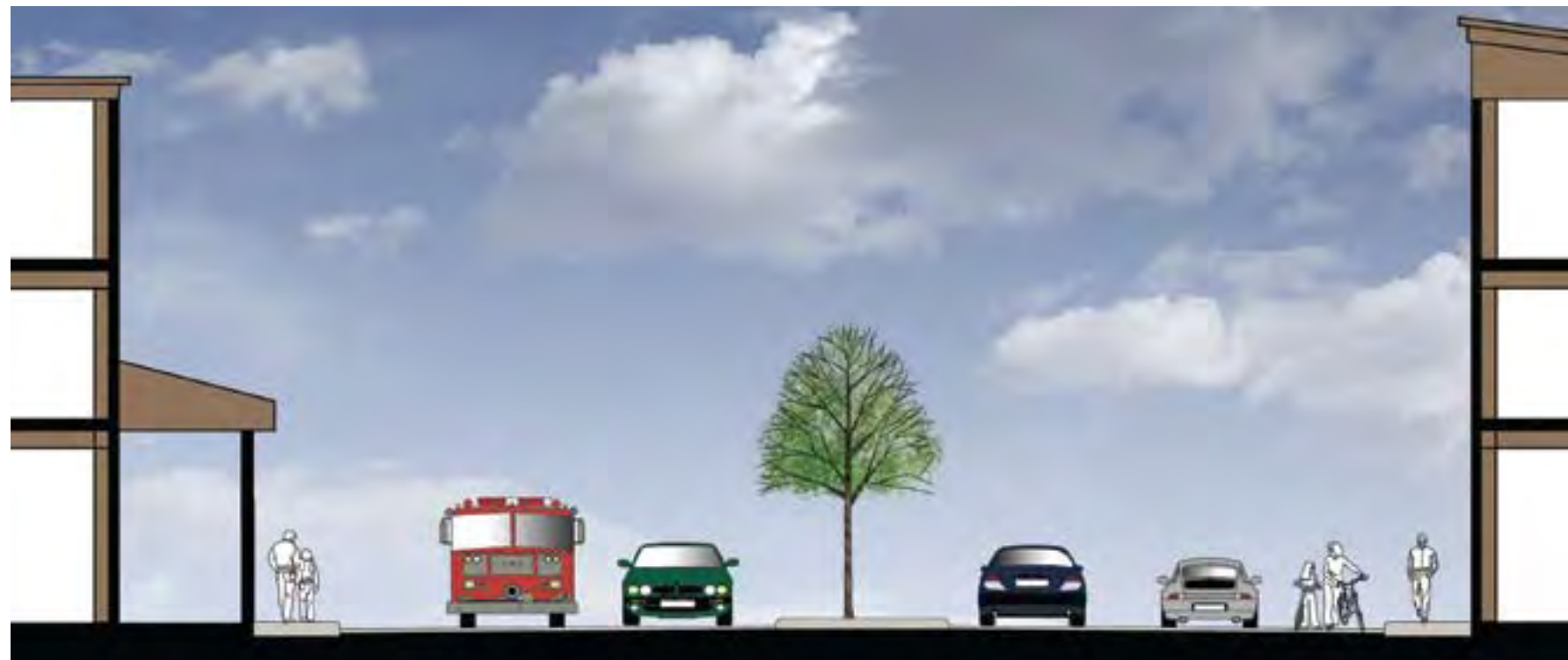
(4) An 80' right-of-way accommodates dual travel lanes and a planted median. A striped bike lane accommodates cyclists through the community center. Pedestrian amenities may be enhanced with widened sidewalks.
