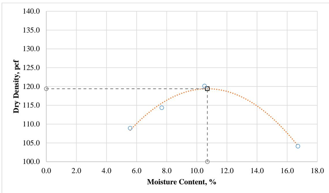
**Figure 89. Moisture-density curve for borrow material (contract 3583).**
