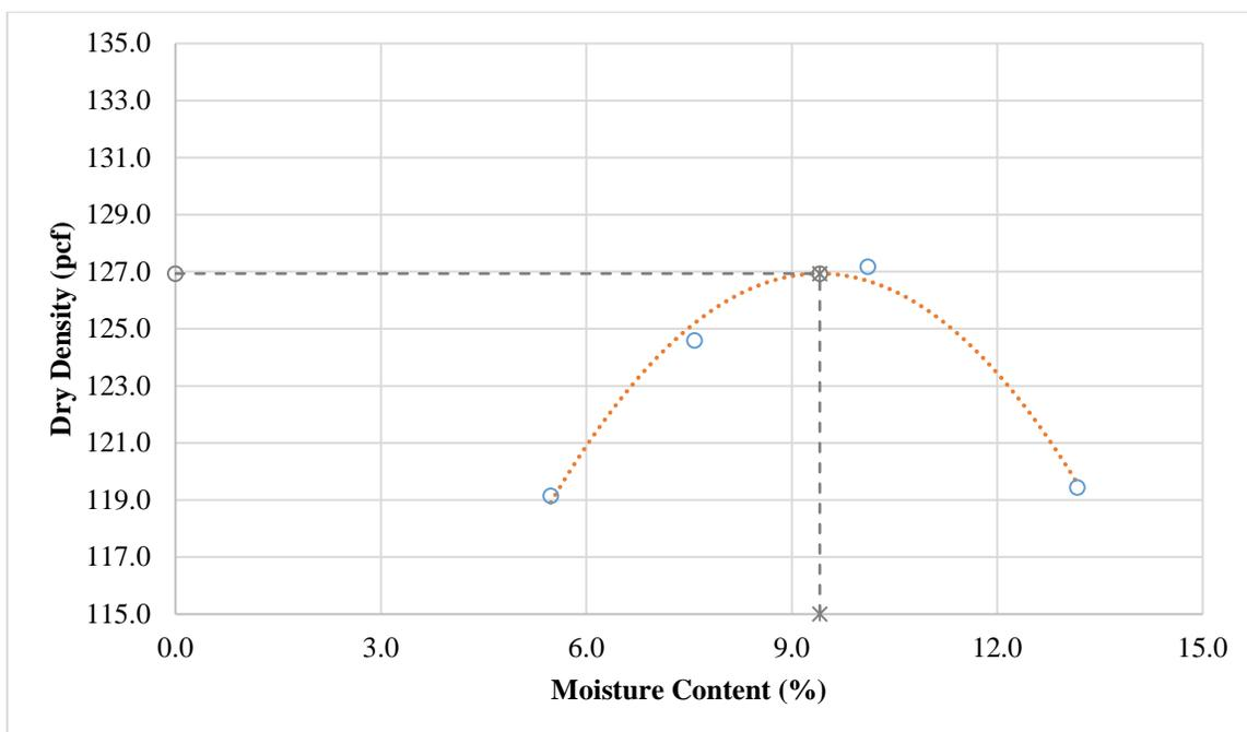
**Figure 94. Moisture-density curve for subgrade material (US-95/Bonnie Claire).**
