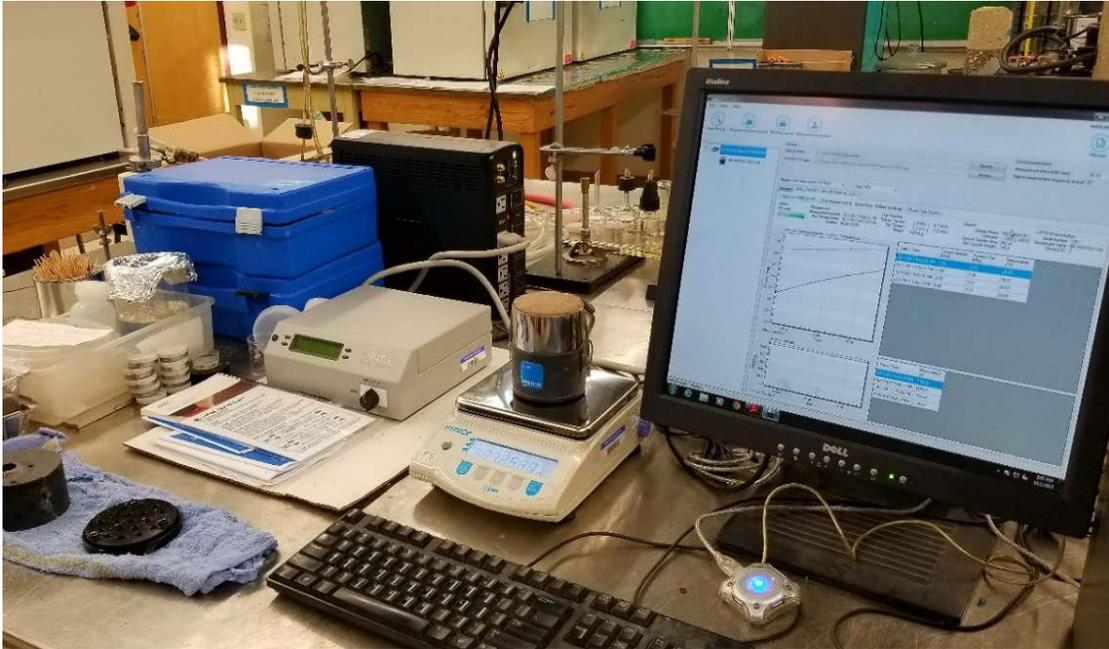
**Figure 39. HYPROP setup.**
