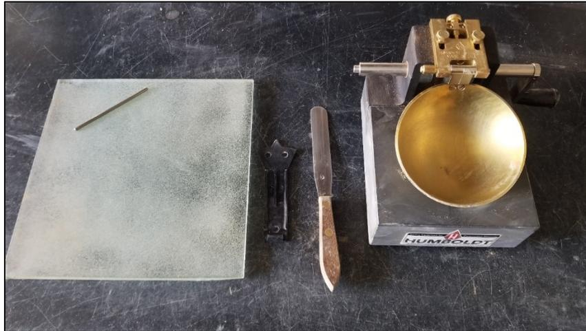
**Figure 33. Atterberg limits testing equipment.**
