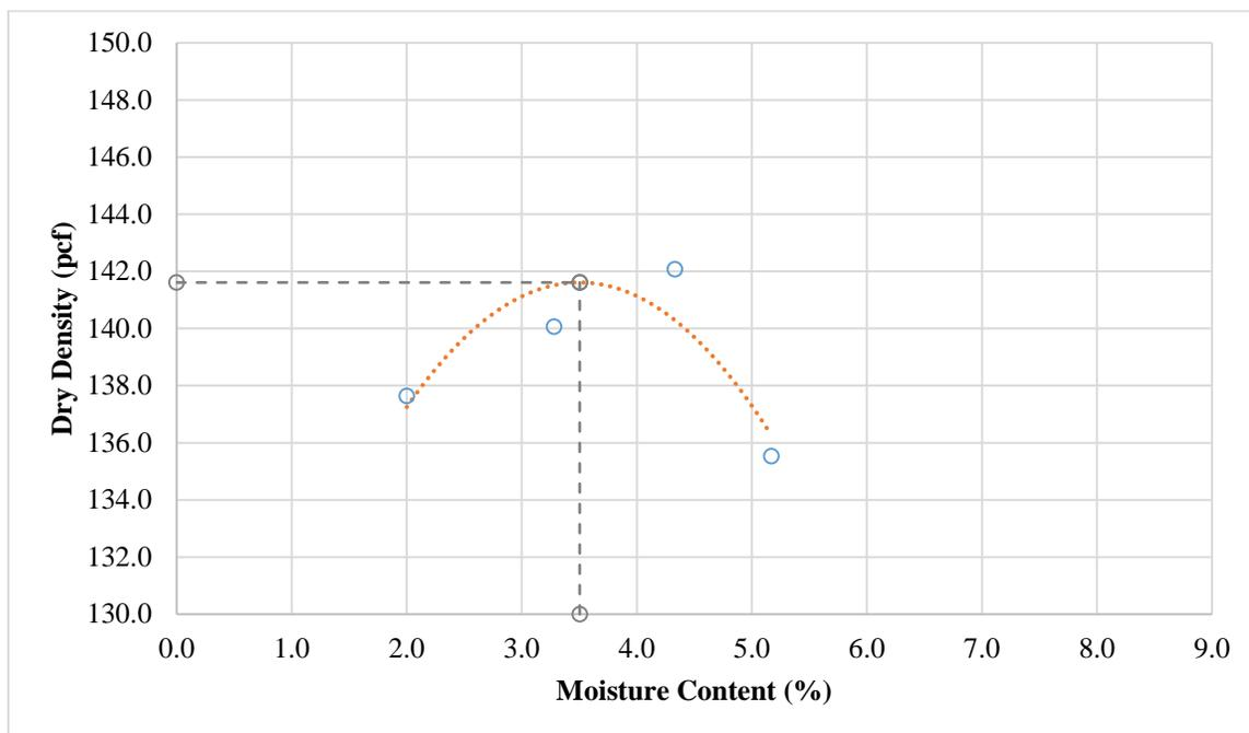
**Figure 87. Moisture-density curve for base material (contract 3613).**
