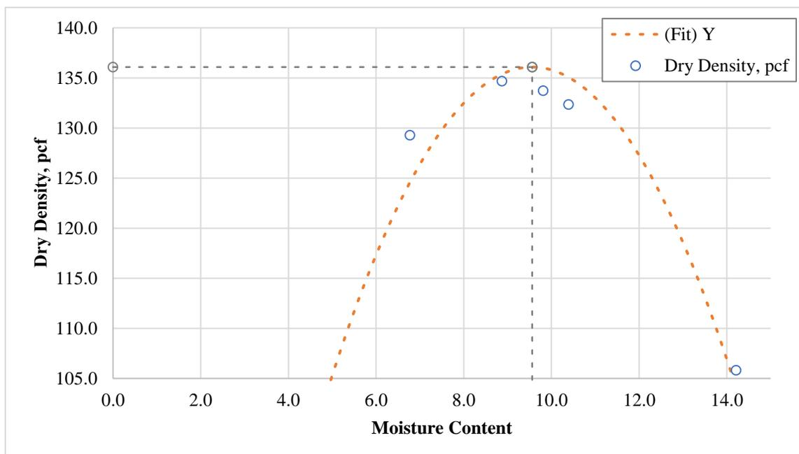
**Figure 100. Moisture-density curve for SNC Secondary borrow.**
