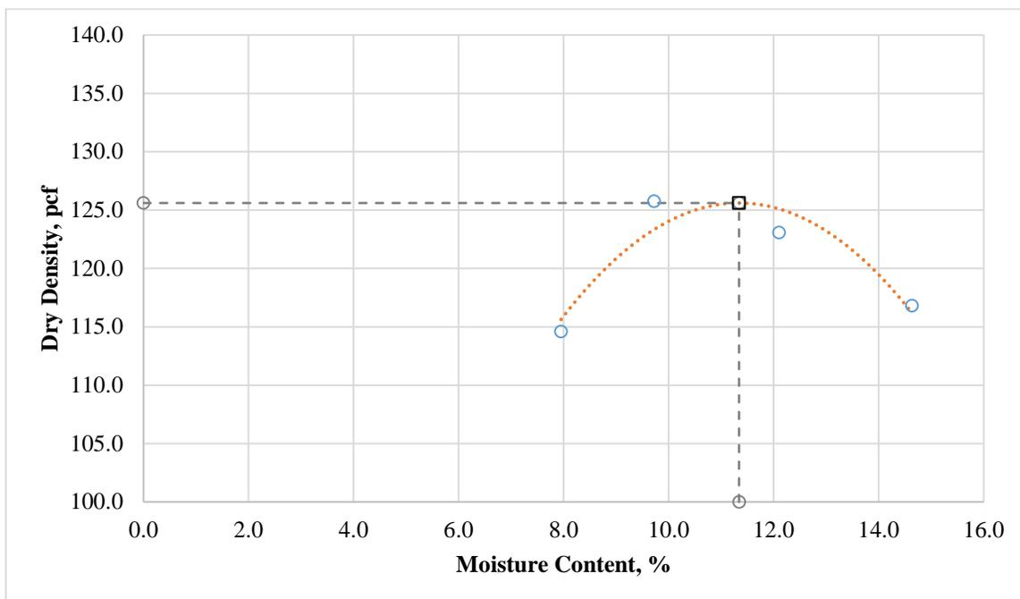
**Figure 91. Moisture-density curve for borrow material (contract 3607).**
