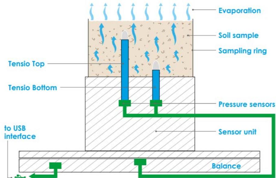
**Figure 6. Diagram of HYPROP – after UMS (12).**
