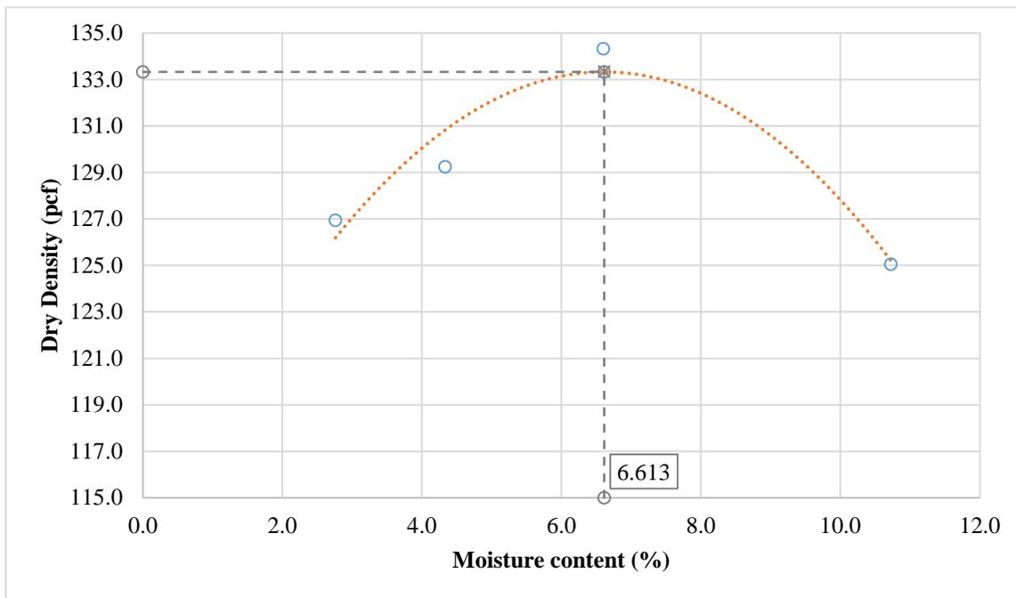
**Figure 93. Moisture-density curve for subgrade material (US-95/Searchlight).**
