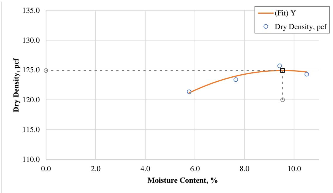
**Figure 105. Moisture-density curve for Elko borrow.**
