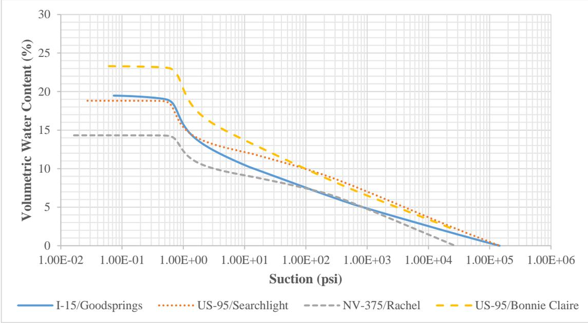
**Figure 63. Subgrade material SWCC (Texas A&M estimation method).**
