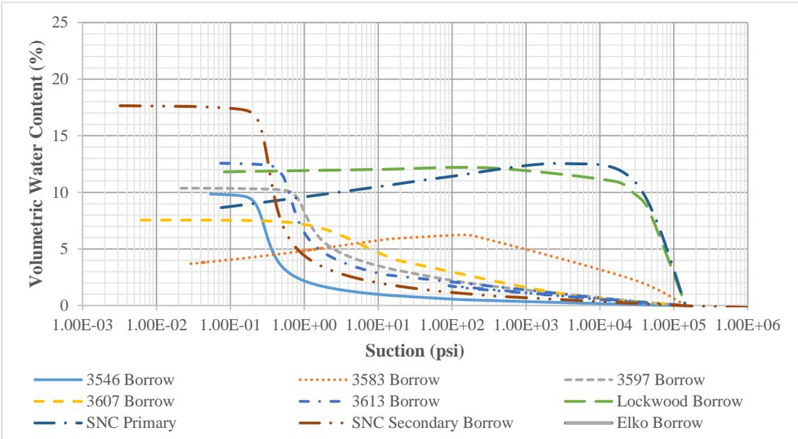
**Figure 60. Borrow material SWCC (input level 2).**
