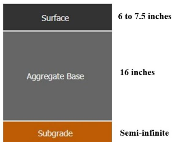
**Figure 64. Pavement design used for sensitivity analysis.**
