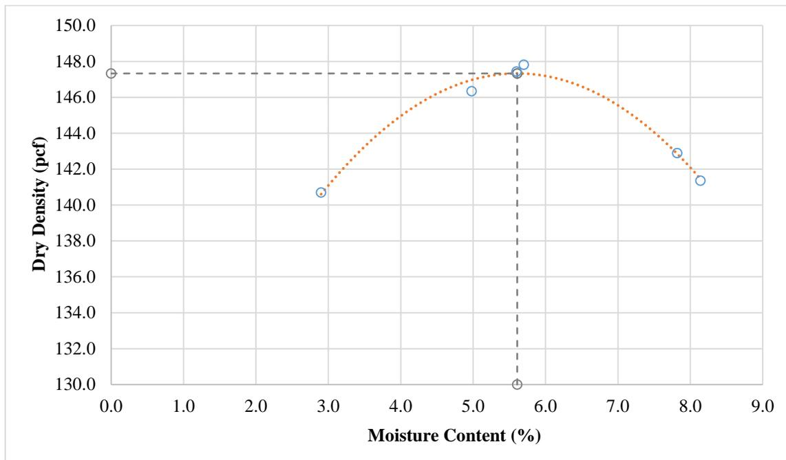
**Figure 83. Moisture-density curve for base material (contract 3583).**
