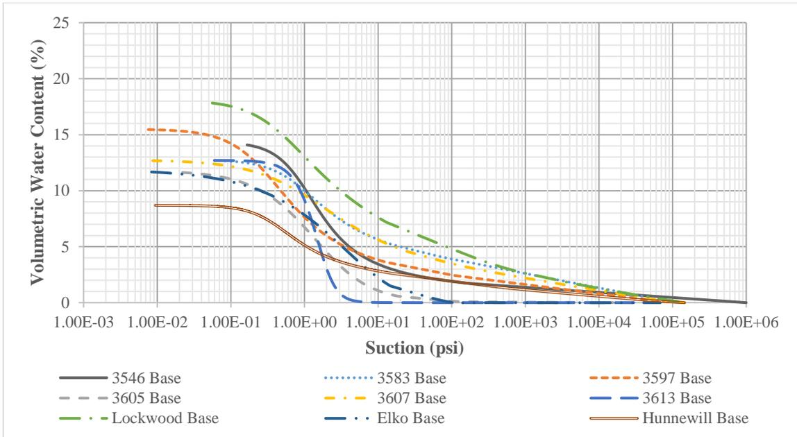
**Figure 56. Base material SWCC (input level 1).**
