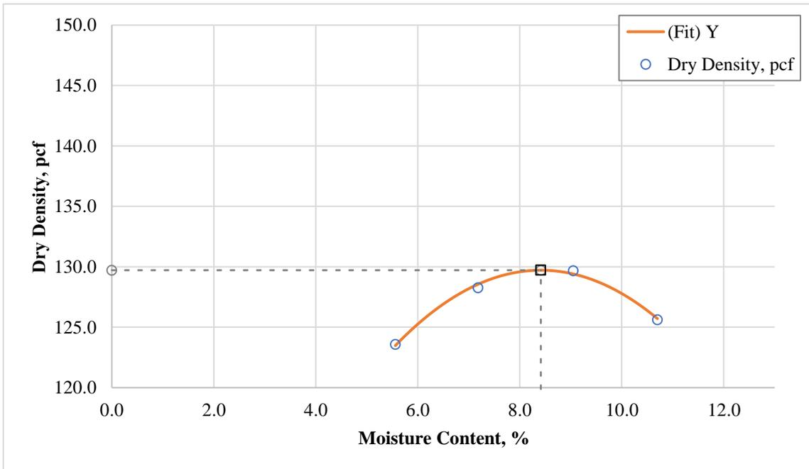
**Figure 104. Moisture-density curve for Elko base.**
