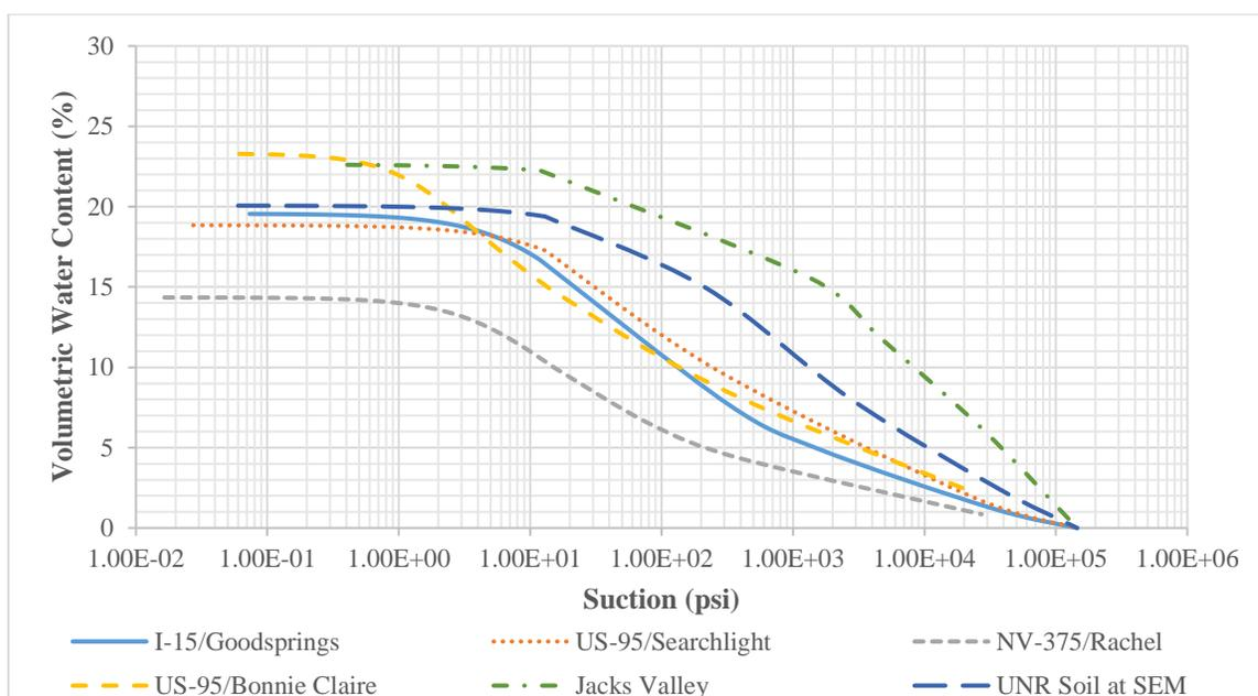
**Figure 61. Subgrade material SWCC (input level 2).**
