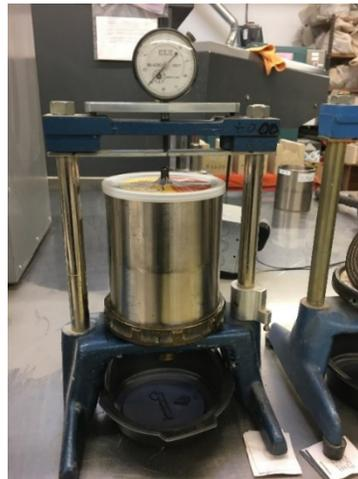
**Figure 45. Expansion pressure device.**
