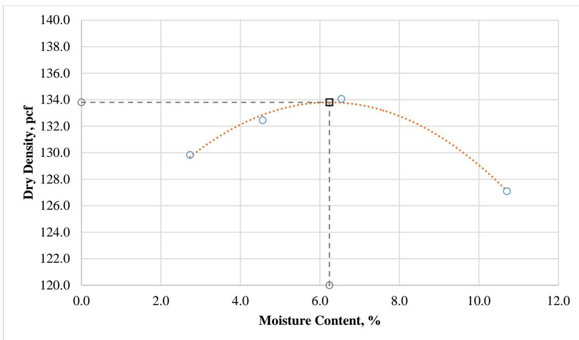
**Figure 90. Moisture-density curve for borrow material (contract 3597).**
