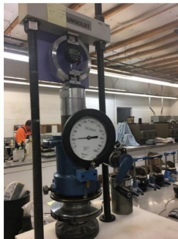
**Figure 46. R-value testing equipment.**
