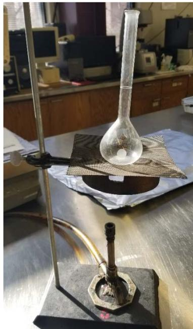
**Figure 36. Soil specific gravity testing equipment.**
