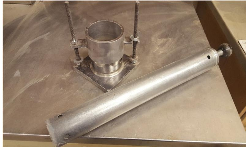
**Figure 38. Compaction equipment for SWCC samples.**
