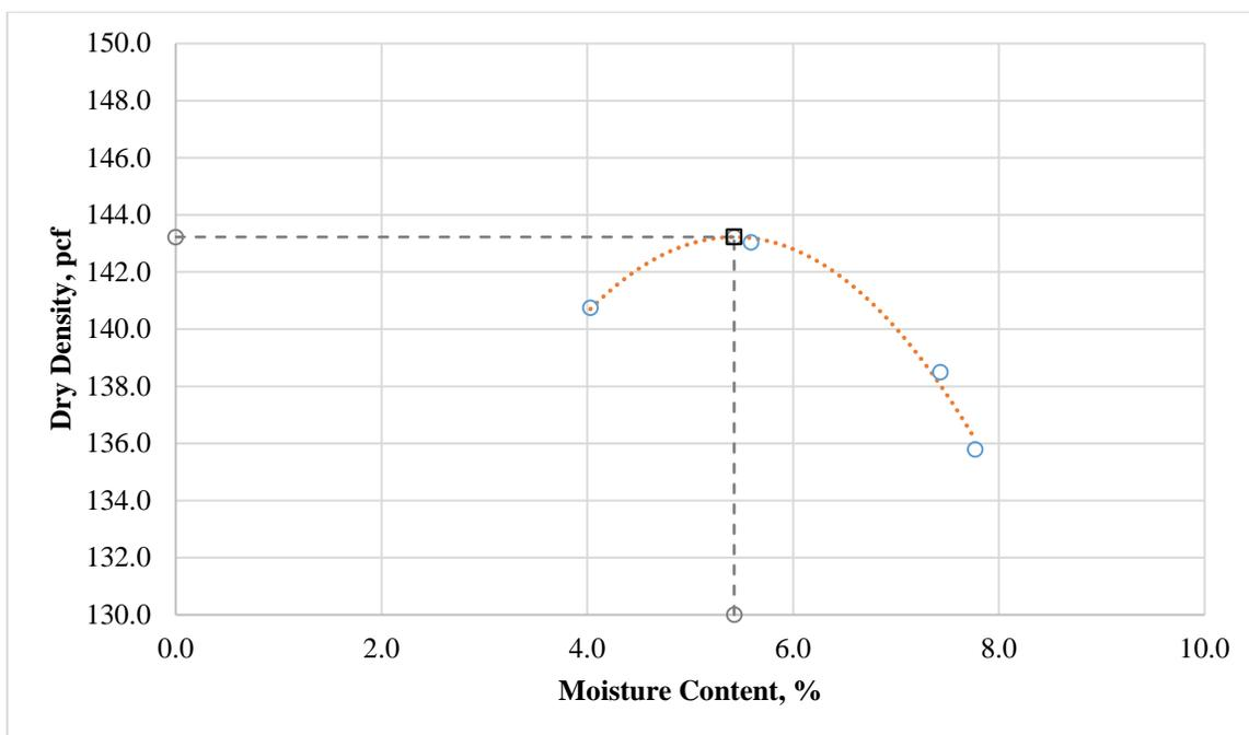
**Figure 92. Moisture-density curve for borrow material (contract 3613).**
