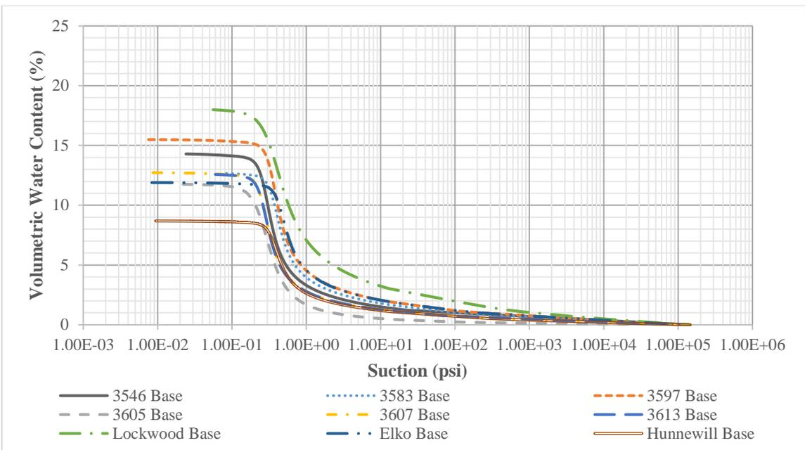
**Figure 59. Base material SWCC (input level 2).**
