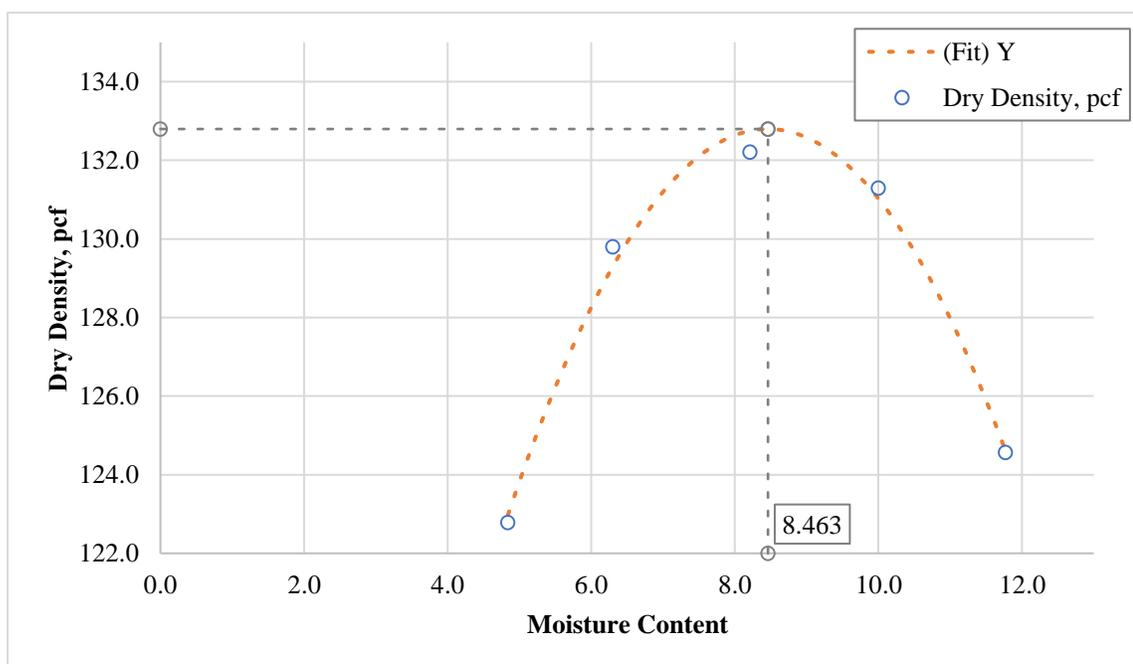
**Figure 102. Moisture-density curve for SEM Soil at UNR.**
