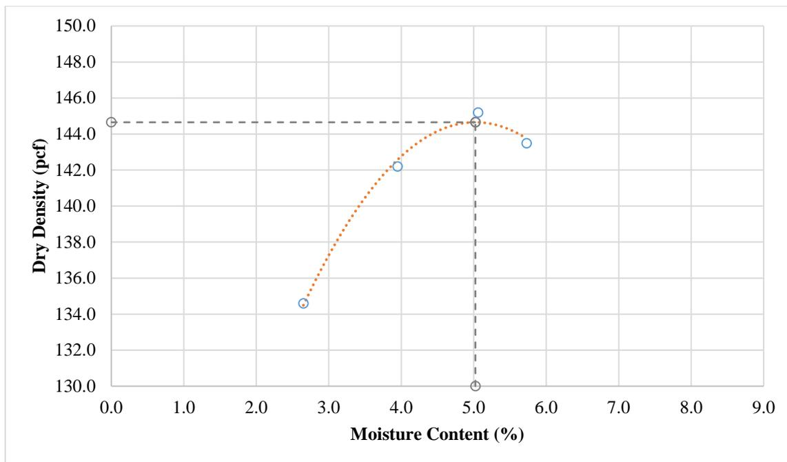
**Figure 82. Moisture-density curve for base material (contract 3546).**
