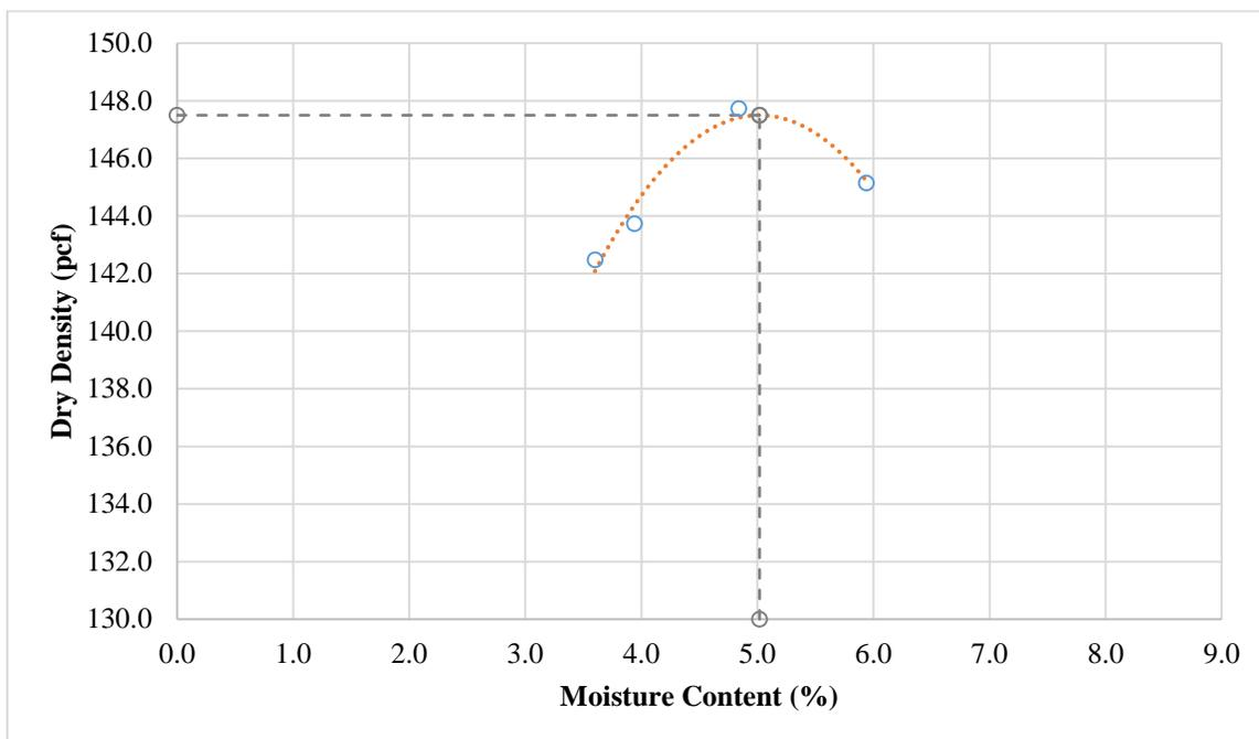
**Figure 85. Moisture-density curve for base material (contract 3605).**
