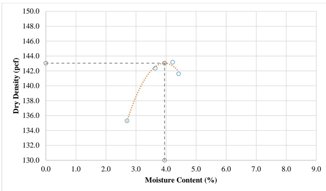
**Figure 84. Moisture-density curve for base material (contract 3597).**
