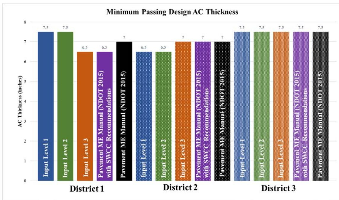
**Figure 78. Minimum passing design AC thickness at each input level.**
