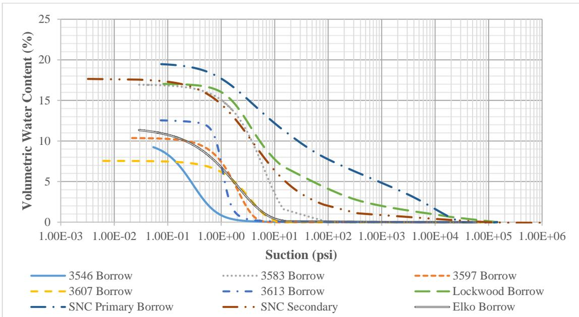
**Figure 57. Borrow material SWCC (input level 1).**
