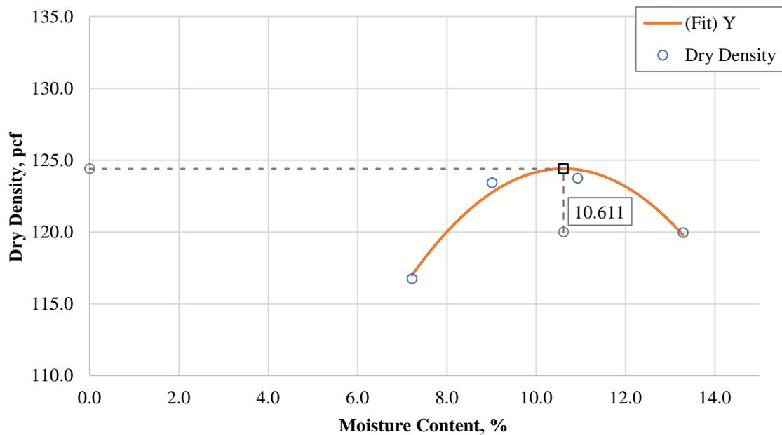
**Figure 99. Moisture-density curve for SNC Primary borrow.**
