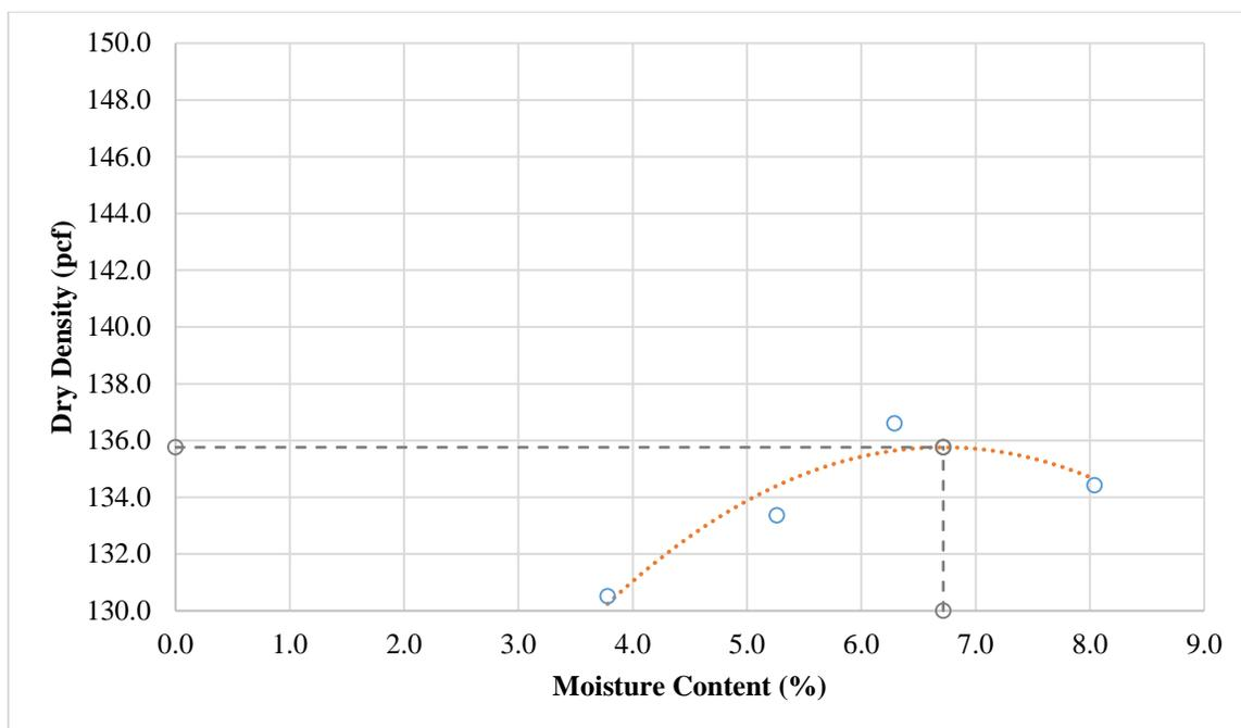
**Figure 86. Moisture-density curve for base material (contract 3607).**
