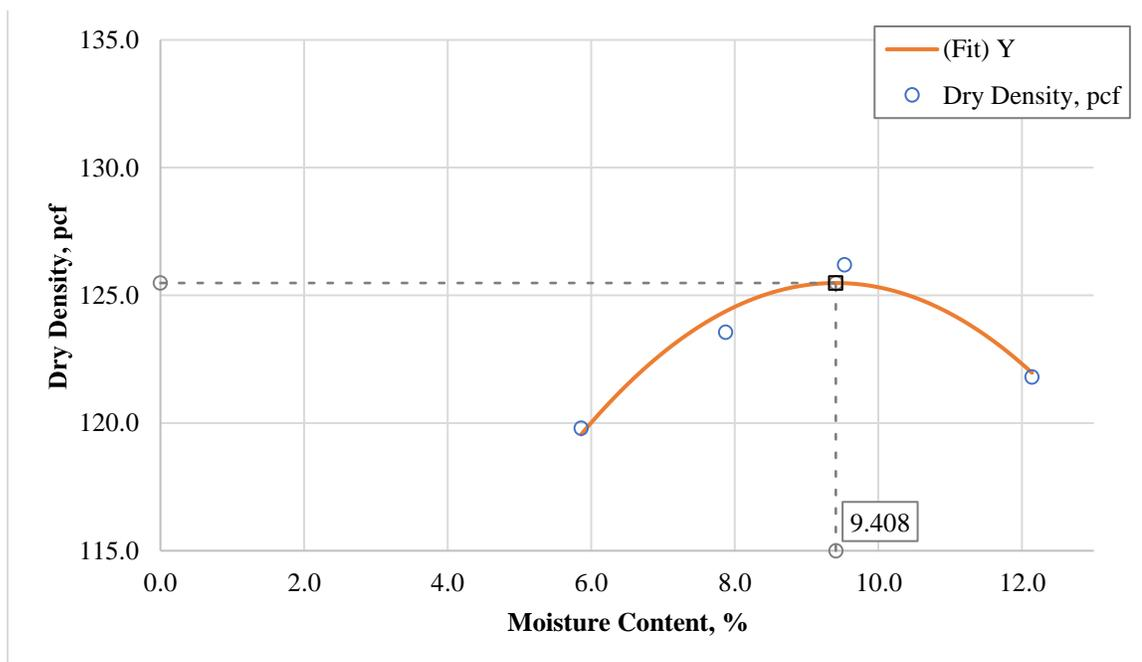
**Figure 101. Moisture-density curve for Jacks Valley subgrade.**
