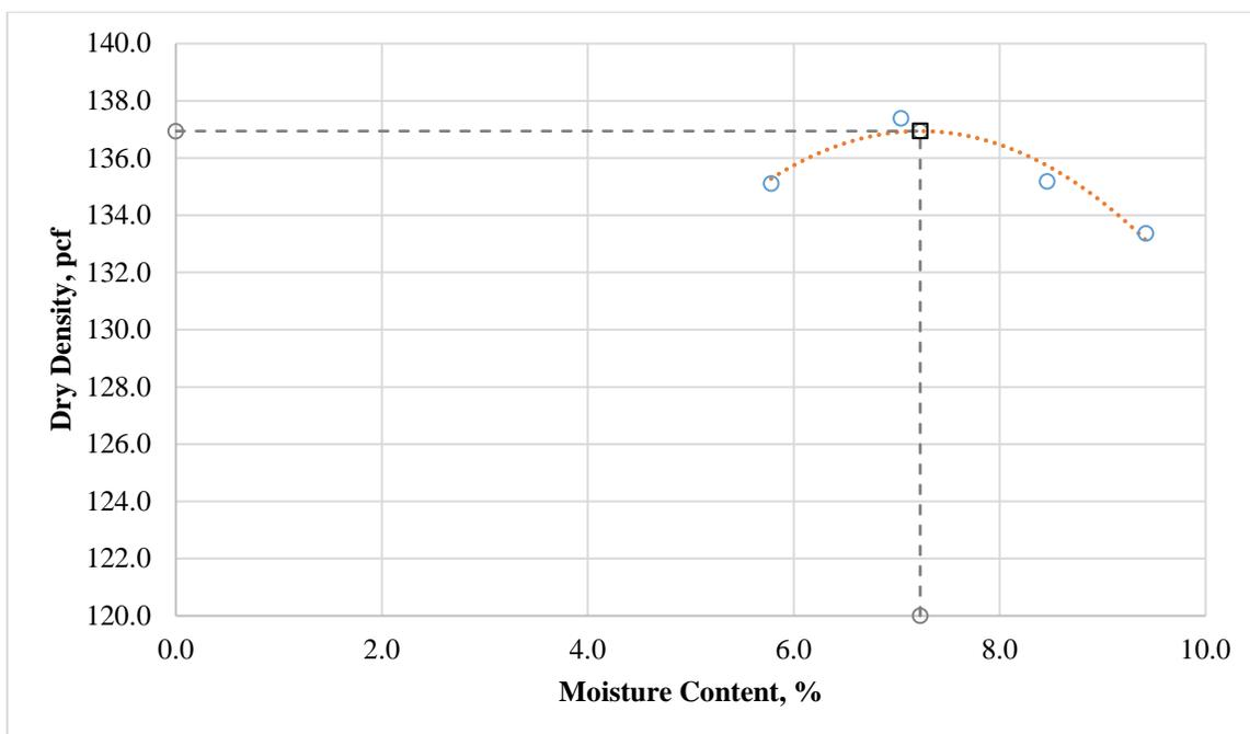
**Figure 88. Moisture-density curve for borrow material (contract 3546).**
