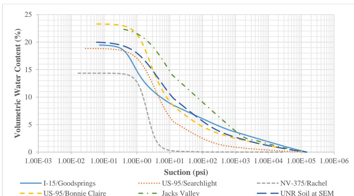
**Figure 58. Subgrade material SWCC (input level 1).**
