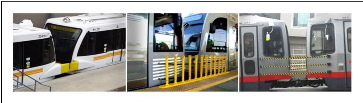
Figure 4-7 – Between-Car Barriers in Light Rail Applications
