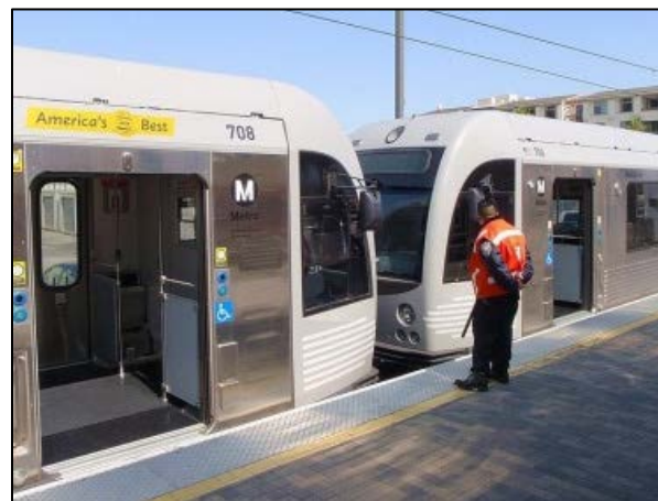
Figure 4-8 – Stationing of Transit Personnel in Lieu of Between-Car Barriers in Light Rail Applications
