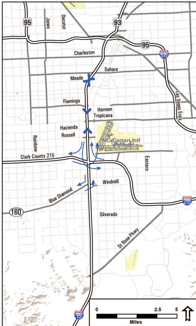
Figure 4-1: Proposed Direct-Access Ramps along I-15
