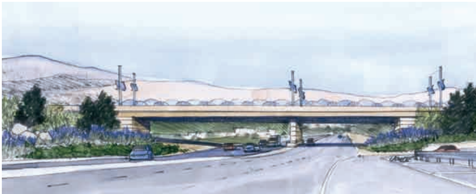
(3) A simplified bridge structure is enhanced through the reduction of slope paving and use of regionally adapted softscape treatments.
