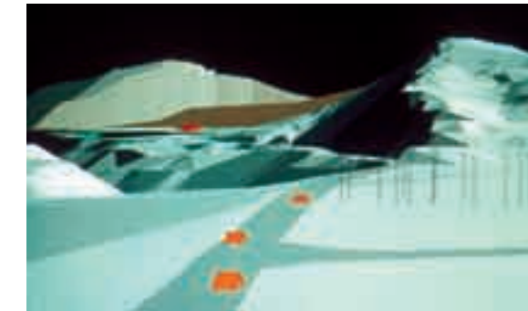
(2) Computer simulation of a planned highway at the conceptualization of the project provides greater understanding of highway layout and potential impacts to environmental resources.
