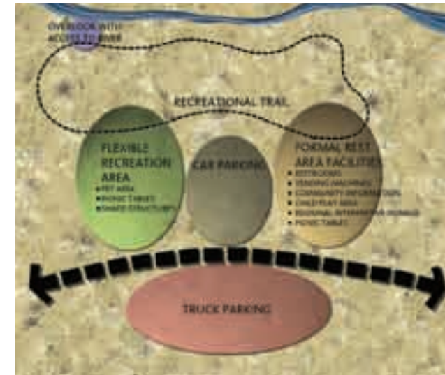
(6) Conceptual layout of rest area amenities responds to environmental context and separates truck parking from view corridors.
