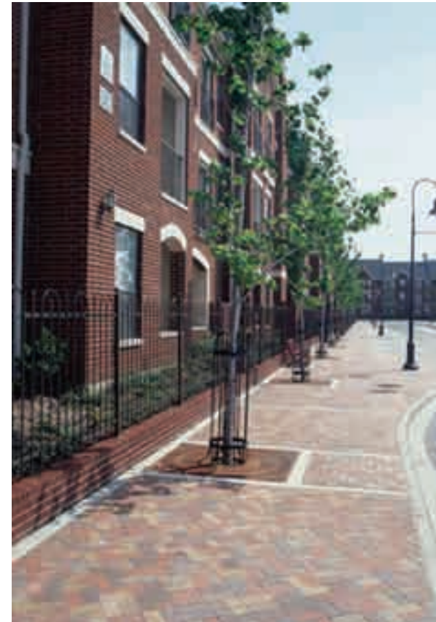
(3) Place street trees where they are protected from car door damage and in areas where they easily facilitate pedestrian movement.
