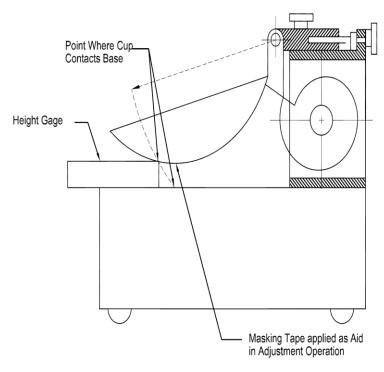
Figure 2—Calibration for Height of Drop
