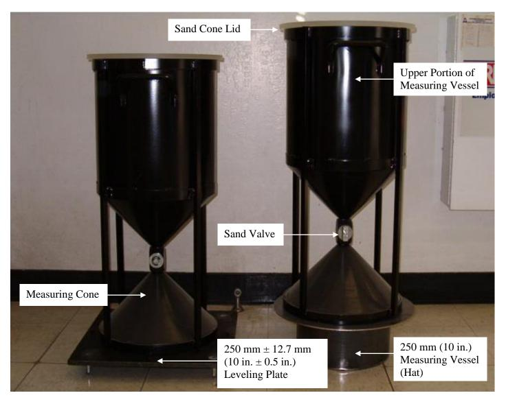
One piece sand cone and 250 mm (10 in.) measuring vessel (hat)
