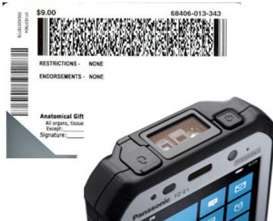
Figure 5. Driver's License Barcode Reader
