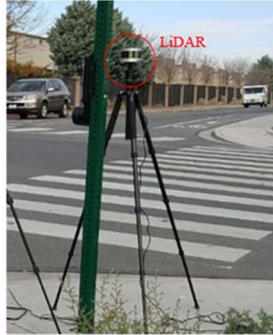
(a) Permanent installation (b) Temporary installation Figure 3-3 Different installation methods of roadside LiDAR sensors
