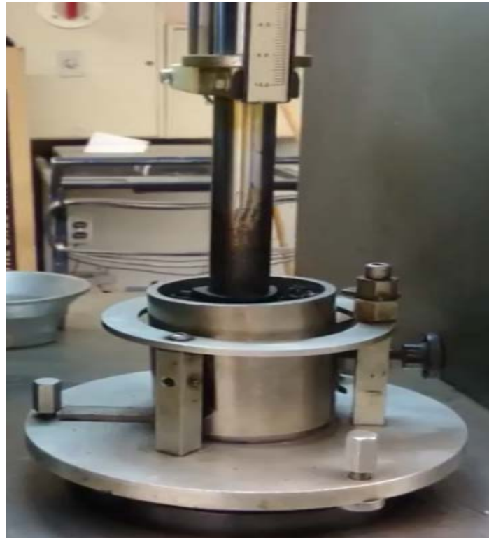
Figure 3.3. Hveem kneading compaction set-up.
