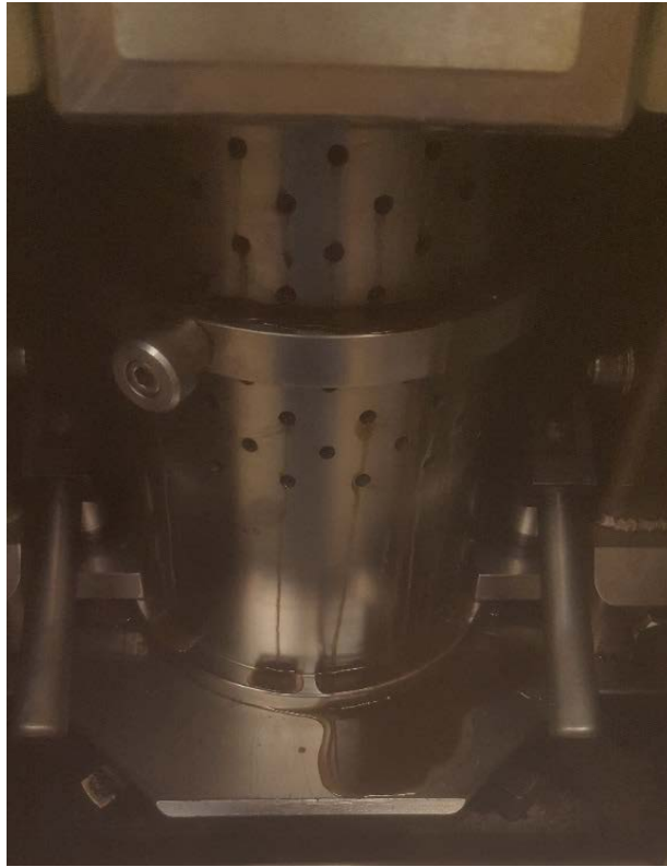
Figure 3.9. SGC perforated mold used in the compaction of CIR mixtures.
