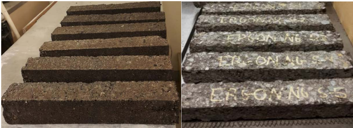
Figure 4.12. Original CIR beams and cut test beams.
