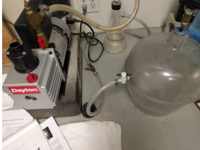
Figure 4-12 Rapid chloride permeability test setup
