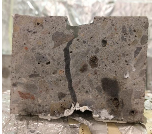
Figure 4-19 Cross section of a specimen filled with crack sealer
