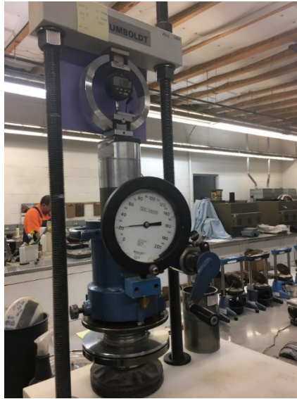
Figure 17. R-value testing equipment.
