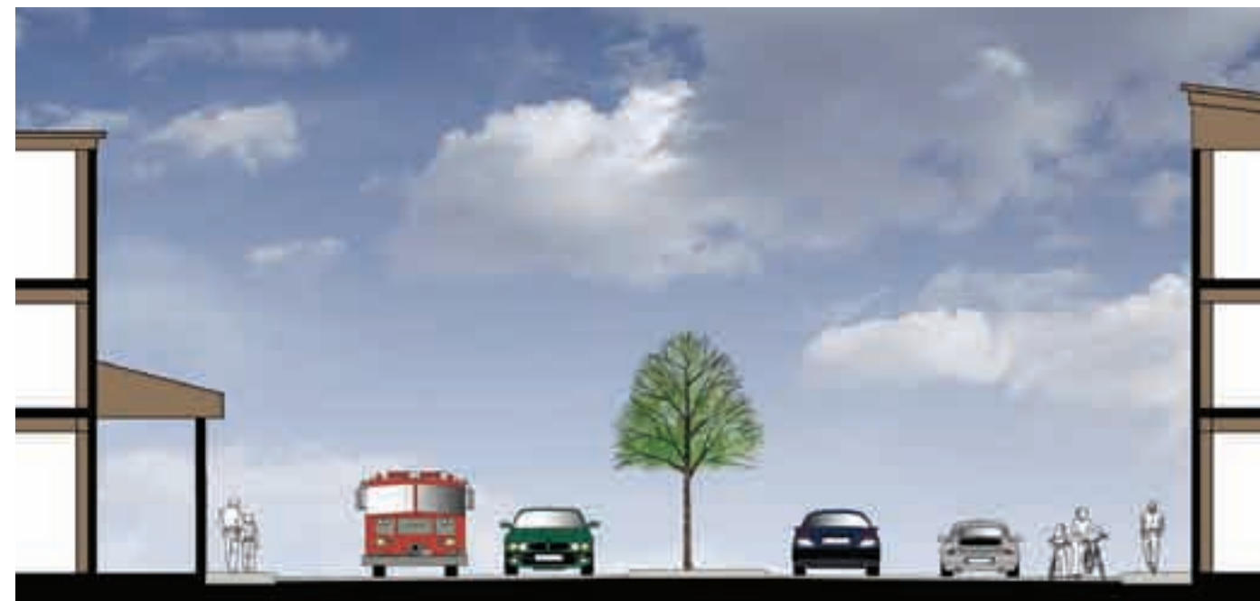
Figure 12 - An 80 foot right-of-way accommodates dual travel lanes and a planted median. A striped bike lane accommodates cyclists through the community center. Pedestrian amenities may be enhanced with widened sidewalks.
