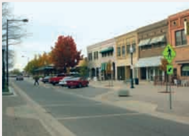
(2) Variations in paving material and color clearly define pedestrian and vehicular circulation zones.
