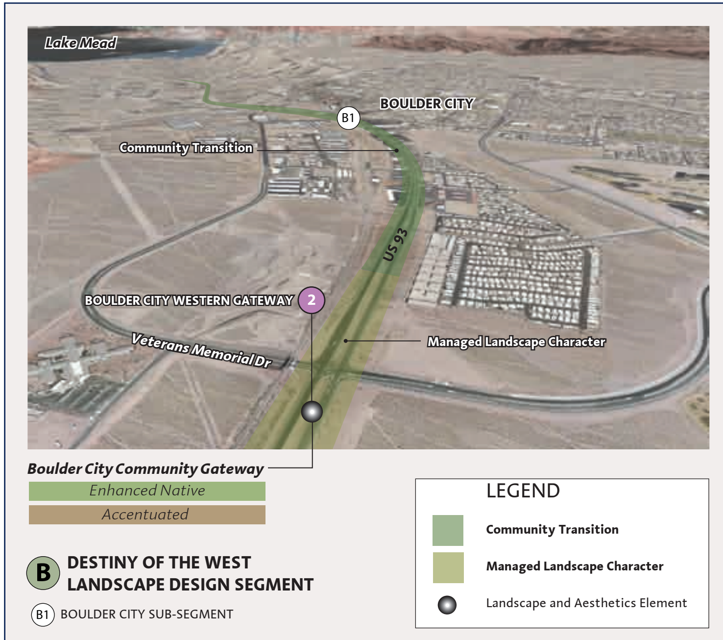
(1) Looking east toward Boulder City from the US 93 intersection with Veterans Memorial Drive. The community gateway is located within the Destiny of the West Landscape Design Segment/Boulder City Sub-Segment and marks the western entrance to Boulder City. As proposed, it will exhibit an enhanced native softscape with an accentuated hardscape treatment.
