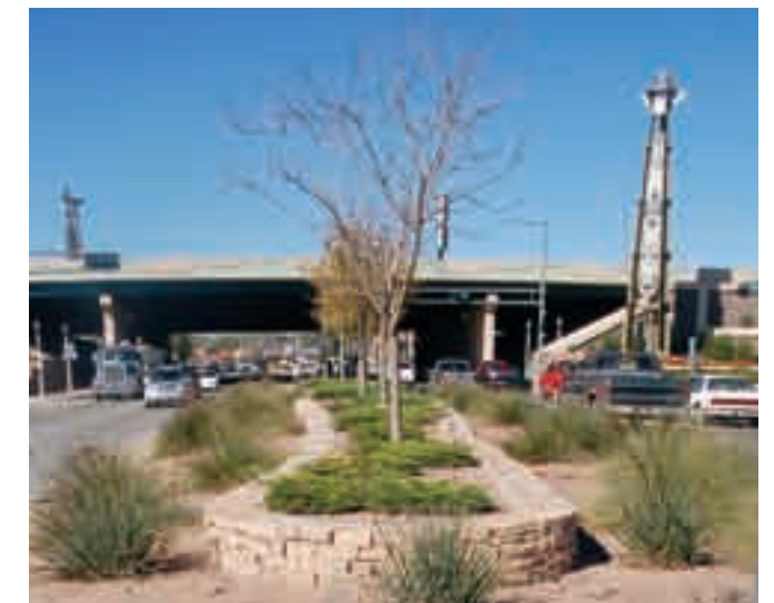
(7) Planted and raised medians help slow traffic through town and create a welcoming environment as travelers enter a community.
