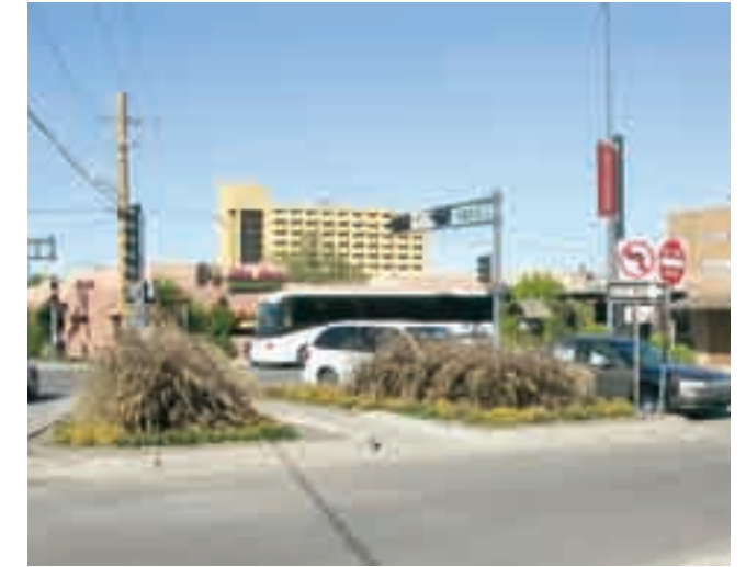
(2) Refuge islands provide a safe place for pedestrians to wait while crossing high traffic areas.
