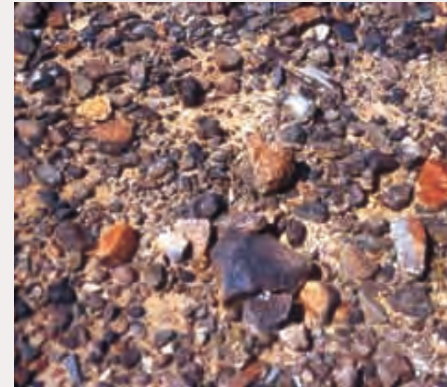
(1) A mix of aggregate size and color helps re-establish disturbed slopes to a naturalized condition.
