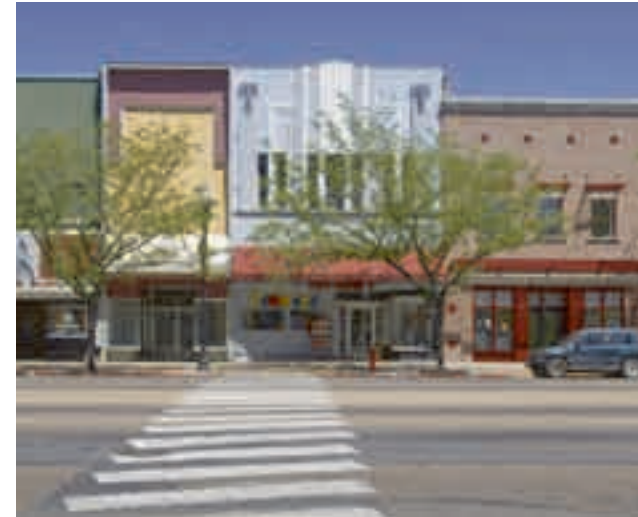
(1) Pedestrian crossings should be visually highlighted with zebra striping or changes in paving type.
