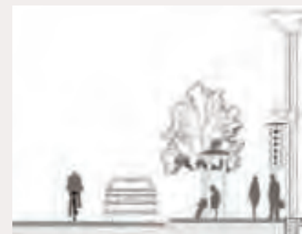
(4) 15 foot sidewalks create space for high levels of pedestrian activity.
