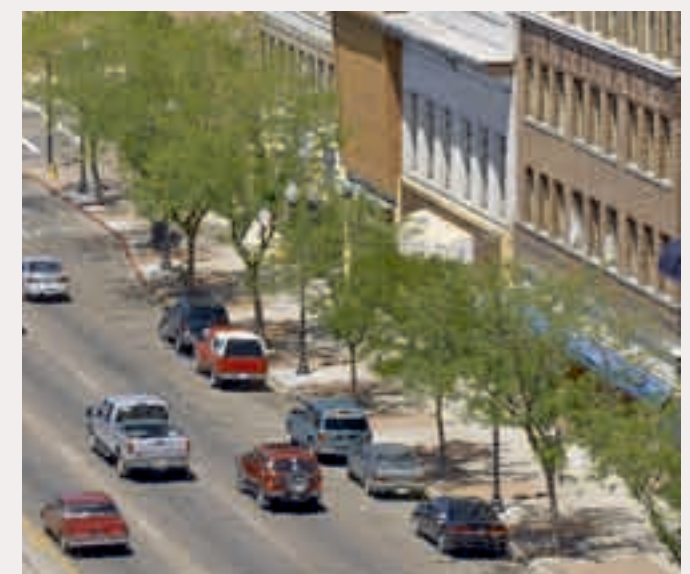
(7) Continuous sidewalks, street trees, and pedestrian amenities are part of a complete main street system that enhances community character and pedestrian safety.
