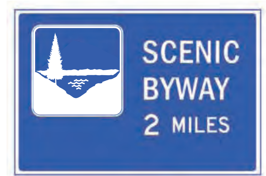
(7) Scenic Byways should include a specific pictorial graphic that is related to the place.
