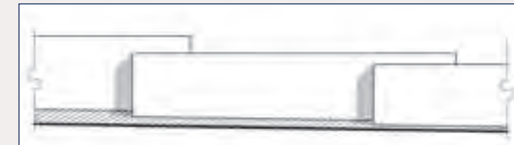
(4) Consider - Stepped transition with staggered walls: Preferred transition for noise wall grade changes. Provide a minimum stagger of 24 inches between wall planes.
