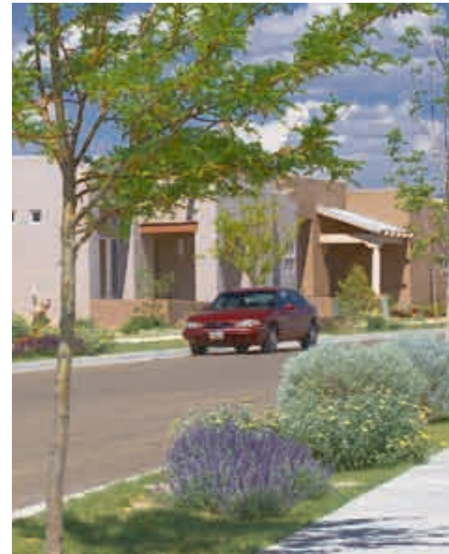
(1) Planting strips (five foot minimum width) provide aesthetic enhancement and increase pedestrian safety by buffering sidewalks from the roadway.
