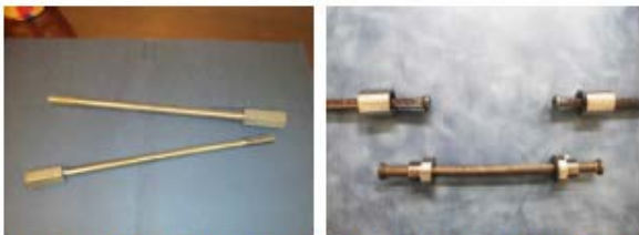
Fig. 6 – CAM bars with threaded couplers (left) and headed couplers (right)
