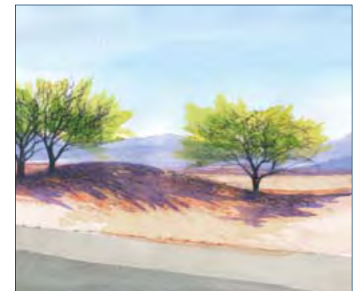
(12) Earth berms or embankment slopes are effective as sound barriers and can be used in combination with partially depressed road profiles. This can avoid walls where sound attenuation is required.
