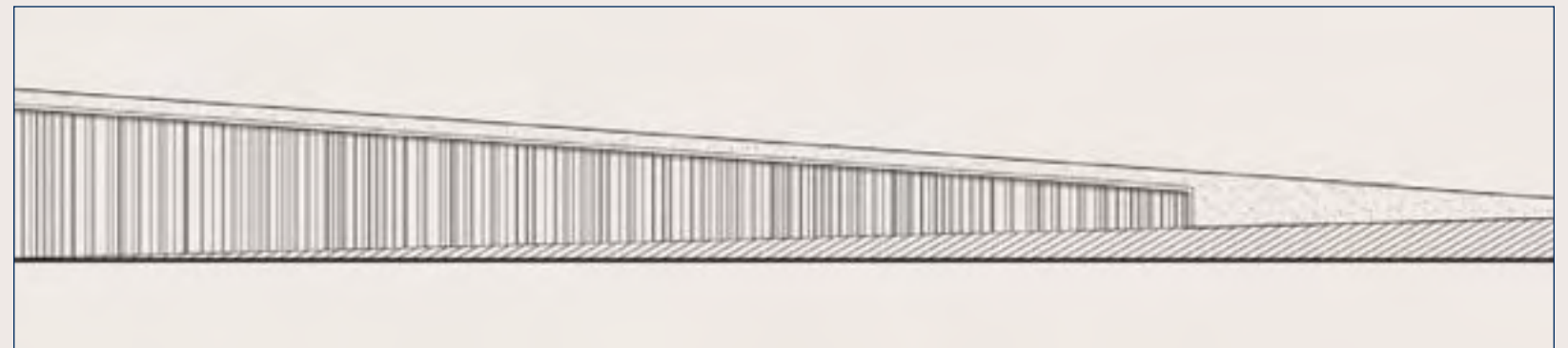
(3) Preferred finish is rusticated variable vertical texture and pattern. Surfaces should have a single finish whether MSE, cast-in-place, or other wall type is used. Consistency with other structures is required.
