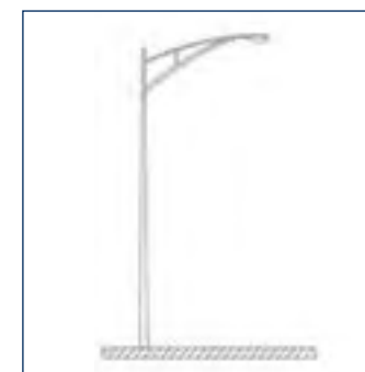
(7) Avoid this type of pole design in favor of more streamlined attachments.
