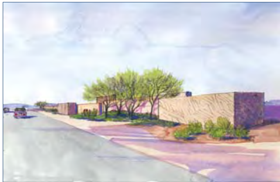
(3), (4), (5) This sequence of travel over approximately 1,000 feet illustrates a prototypical sound wall design for the corridor. Characteristics include staggered wall planes, landscape planting in front of the wall face, and patterning on the wall face.
