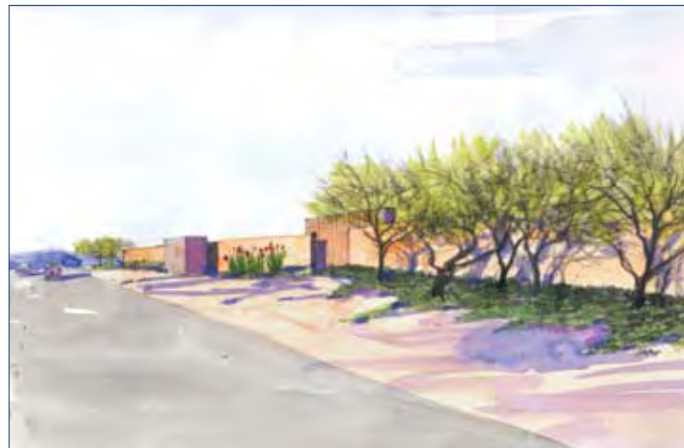
(3), (4), (5) This sequence of travel over approximately 1,000 feet illustrates a prototypical sound wall design for the corridor. Characteristics include staggered wall planes, landscape planting in front of the wall face, and patterning on the wall face.
