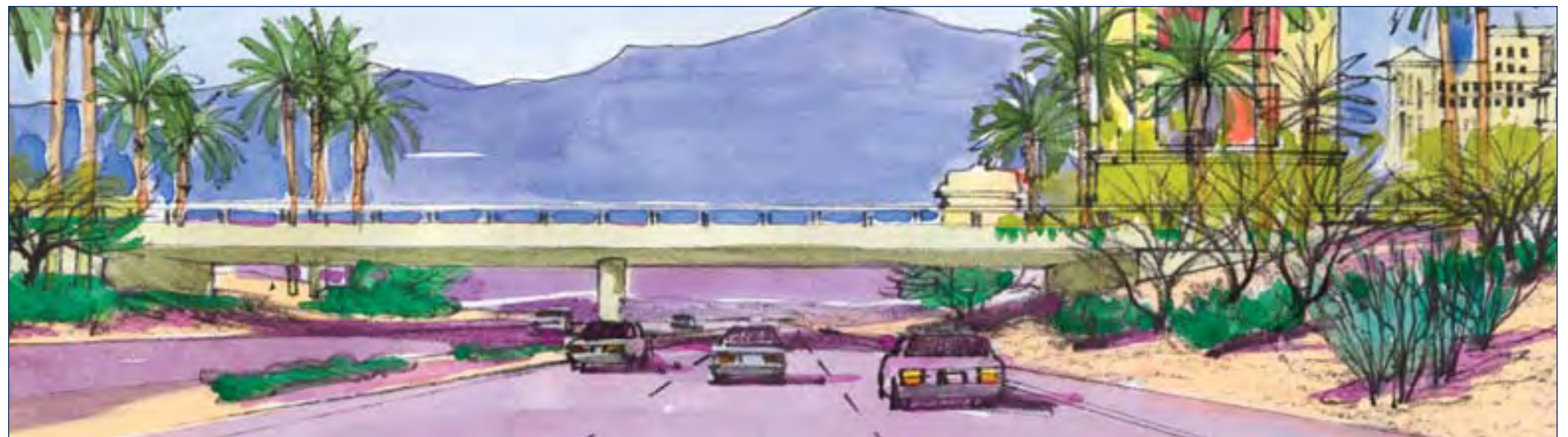
(1) This is an example of Regional Ornamental softscape type planting at the embankment of a highway bridge using the same plants listed in the plant palette above. This type of softscape is limited to the Las Vegas "Flamboyant Resort Corridor."
