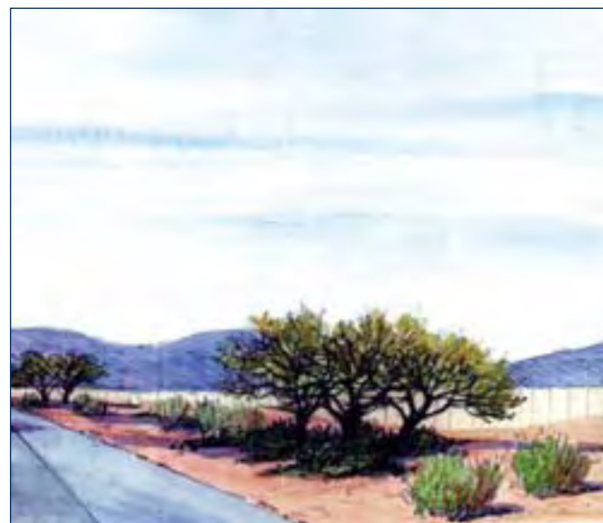
(10) Integrate sound walls into highway right-of-way with landscape planting between wall and roadway. The setback also allows earth contour grading to vary the wall heights and base grade.
