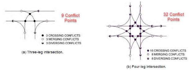
Figure (a) shows 9 conflict points for a 3-Leg intersection or T Intersection. The US 50 corridor will be constructed with alternating T-intersections, to accommodate as much access as possible.
