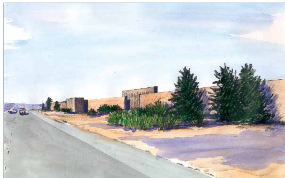
(3) This sequence of travel over approximately 1000 feet illustrates the sound wall design for the corridor. Characteristics include staggered wall planes, landscape planting in front of the wall face, and patterning on the wall face.
