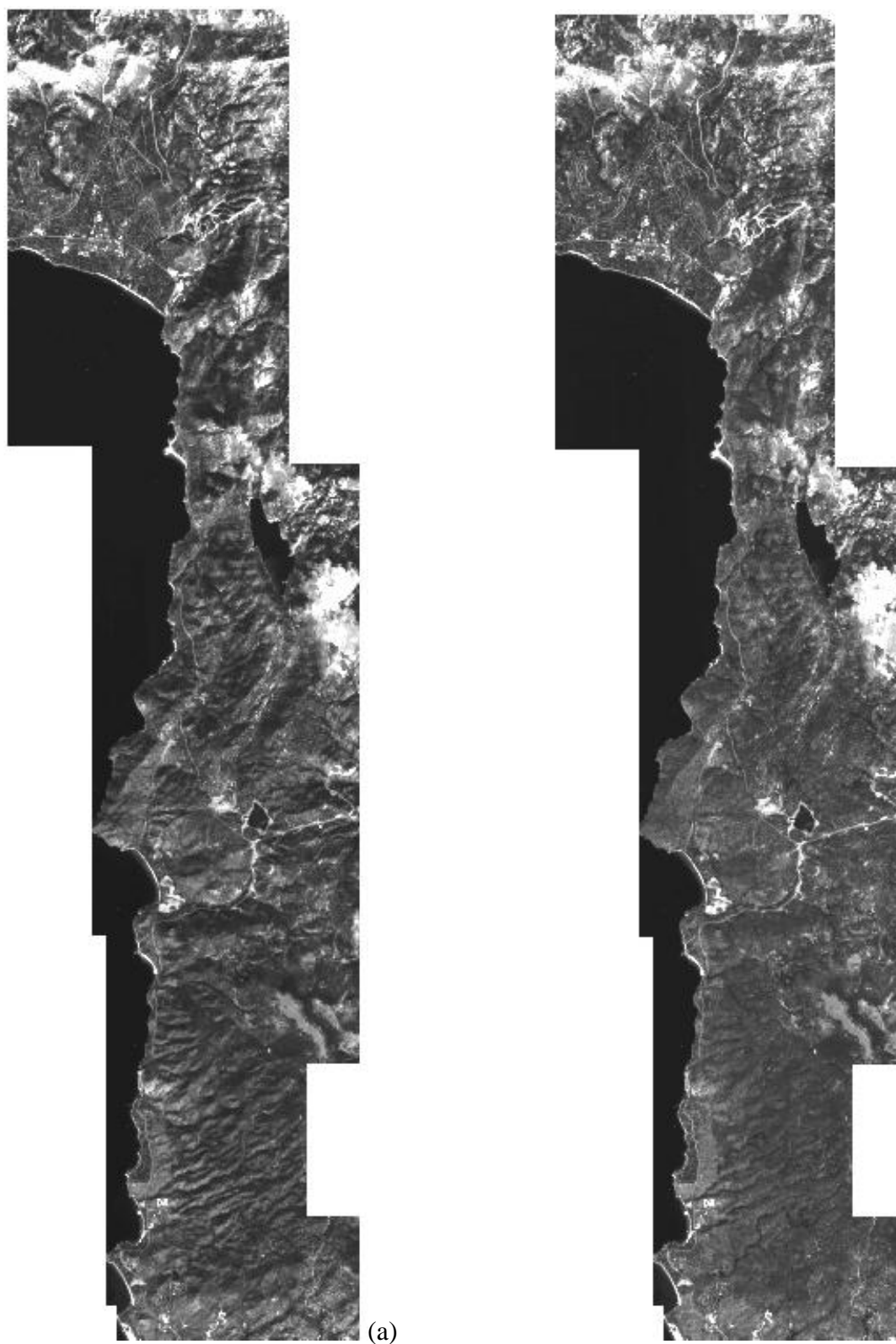
Figure F. 1. The Sun-Crown-Sensor + C topographic correction on the red band of the 27 Sep. 2009 IKONOS image: (a) before correction, (b) after correction.
