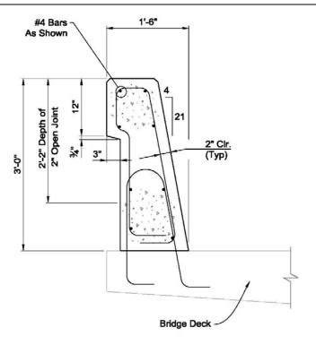
36" Concrete Single Slope Bridge Rail Typical Section Figure 16.5-B
