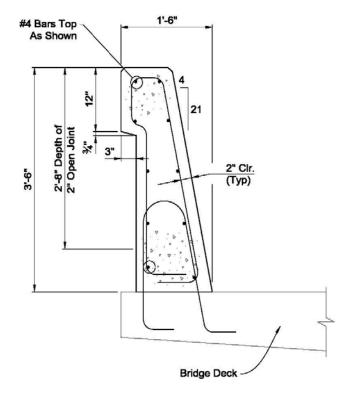
42" Concrete Single Slope Bridge Rail Typical Section Figure 16.5-C
