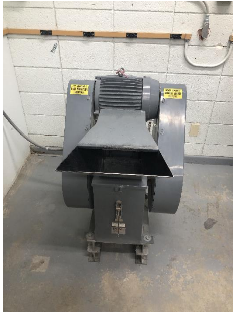
Figure 2.3: Equipment (badger crusher) used to crush the coarse aggregate in to smaller sizes
