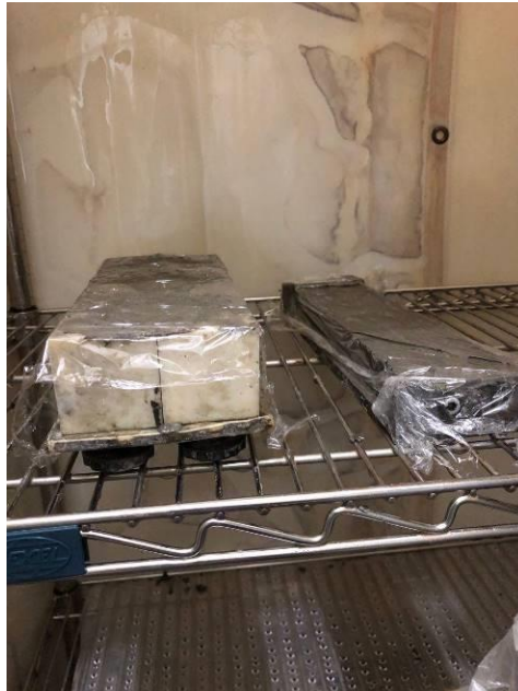
Figure 2.12: Specimens in curing chamber
