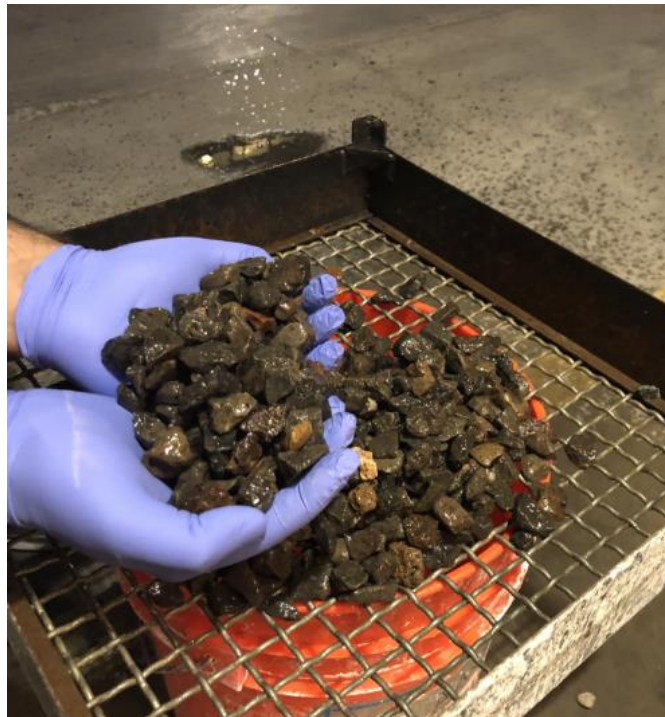
Figure 2.2: Washing coarse aggregates
