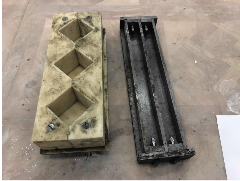
Figure 2.11: Mortar cube and bar molds
