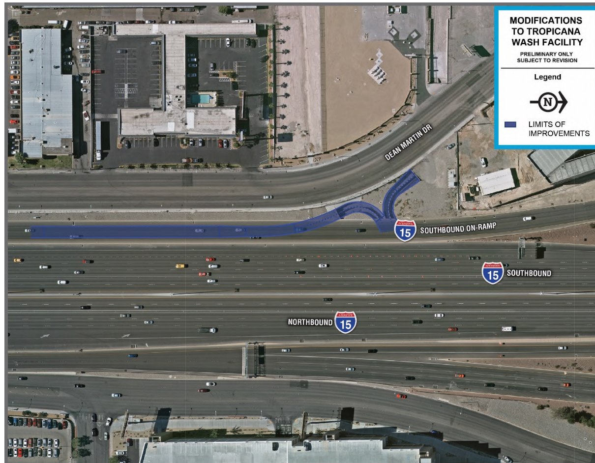
Figure 3-16. Modifications to Tropicana Wash Facility
