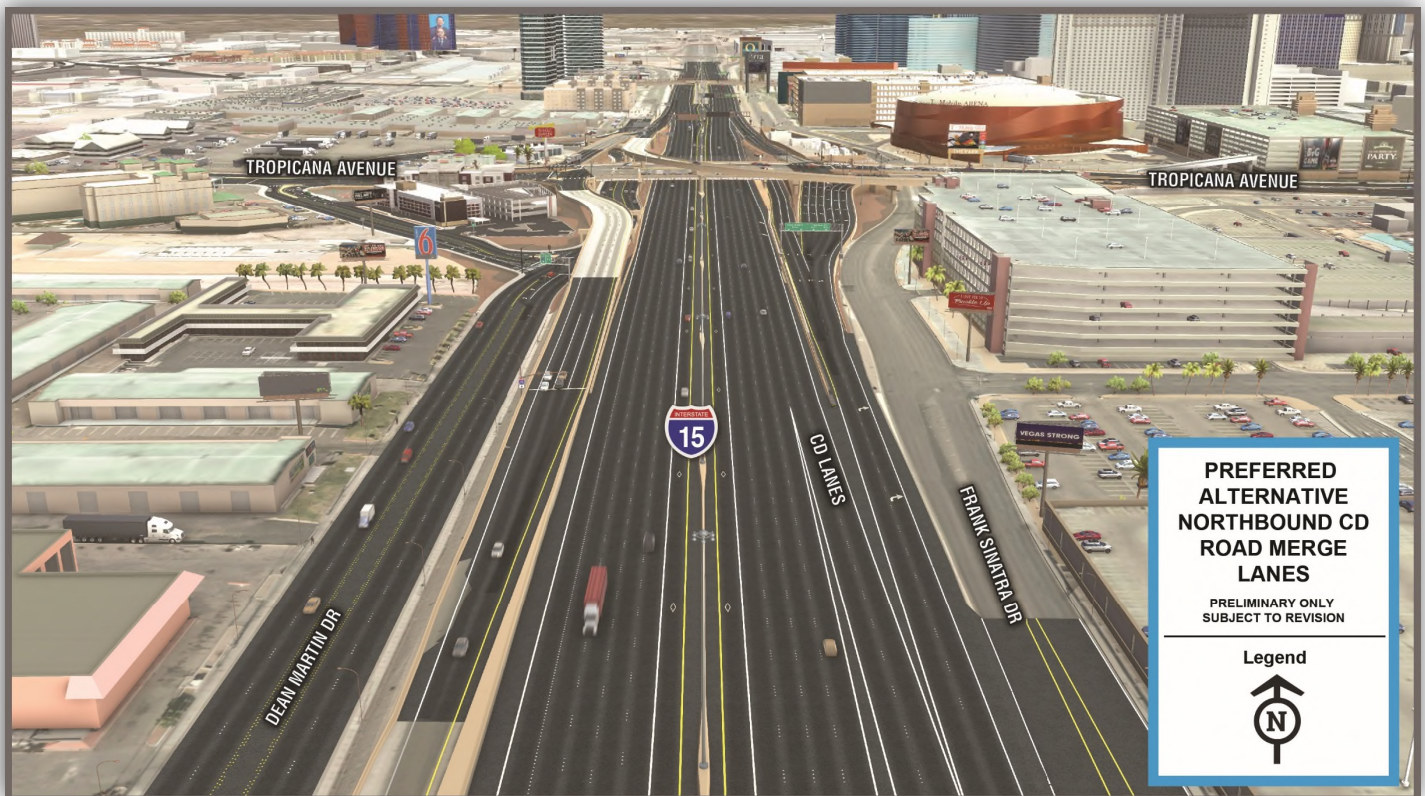
Figure 2-10. Preferred Alternative Northbound CD Road Merge Lanes
