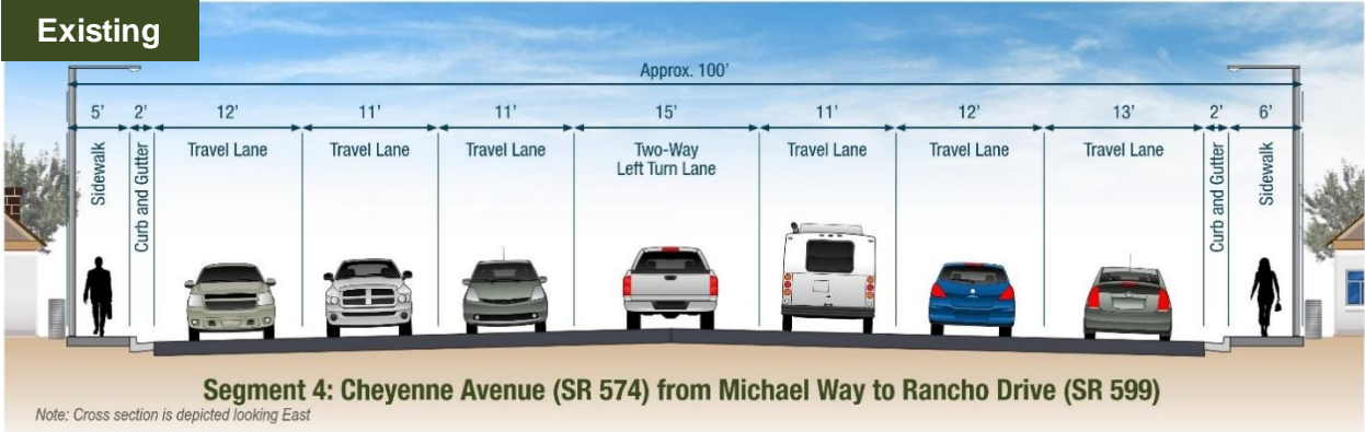
Figure 89 – Cheyenne Avenue (SR 574) Segment 4 Existing Cross Section
