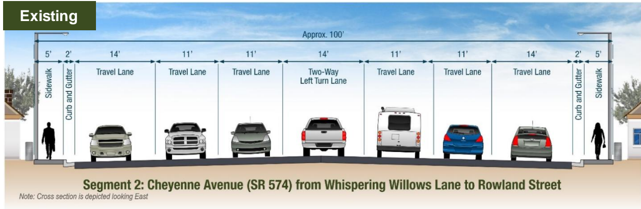
Figure 96 – Cheyenne Avenue (SR 574) Segment 2 Existing Cross Section
