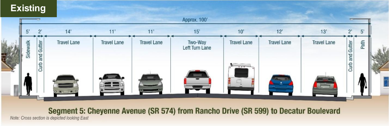
Figure 113 – Cheyenne Avenue (SR 574) Segment 5 Existing Cross Section
