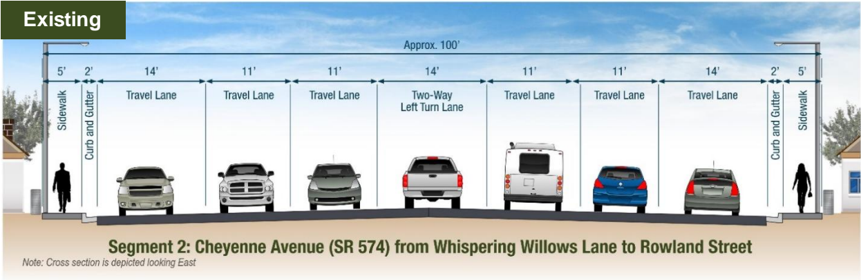
Figure 85 – Cheyenne Avenue (SR 574) Segment 2 Existing Cross Section
