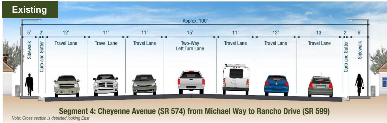
Figure 100 – Cheyenne Avenue (SR 574) Segment 4 Existing Cross Section
