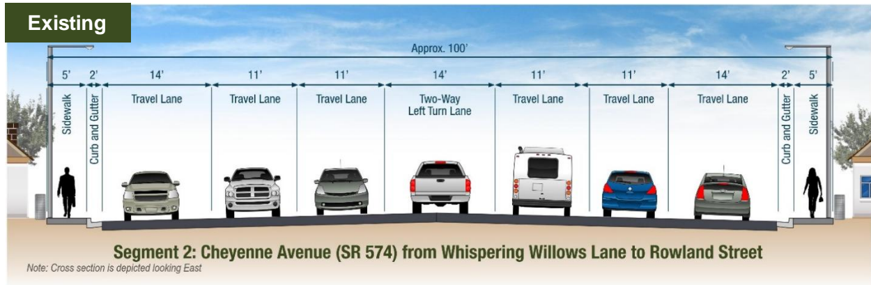
Figure 107 – Cheyenne Avenue (SR 574) Segment 2 Existing Cross Section
