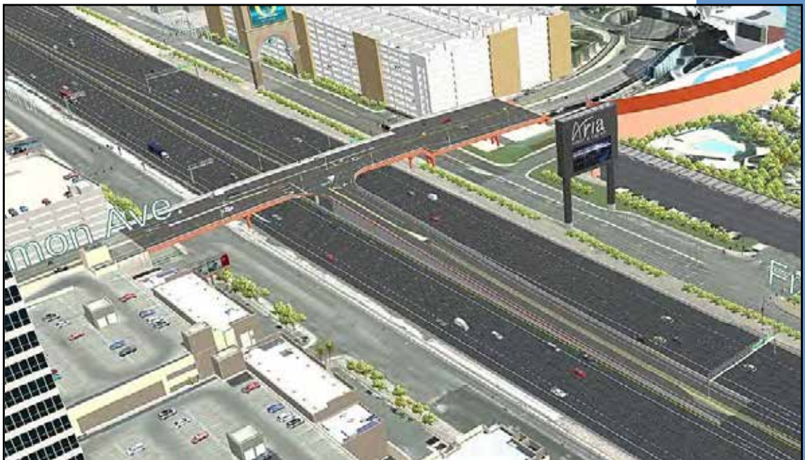
View of the Harmon HOV ramps connecting from I-15 to the south side of the existing Harmon Avenue overpass.
