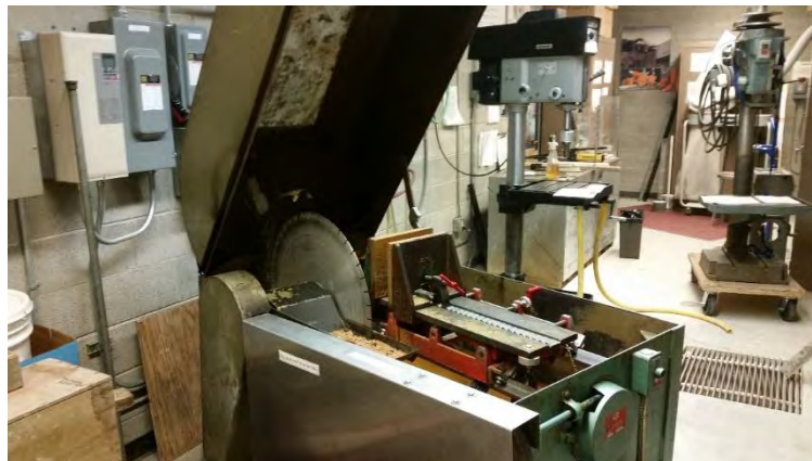
Figure 3.8: Photograph of the diamond core saw used in cutting the cores.
