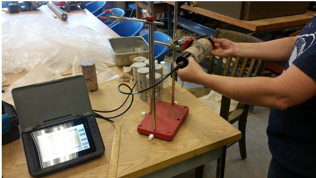
Figure 3.12: Ultrasonic testing configuration.
