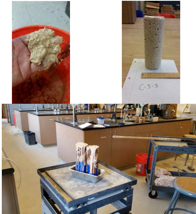
Figure 3.11: Process used to make a reconstituted cemented soil sample.
