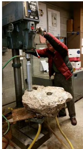
Figure 3.7: Use of the drill press to core cemented soil samples.
