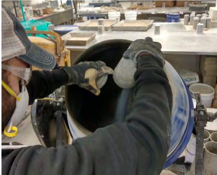
Figure 5.1 Loading silica fume
