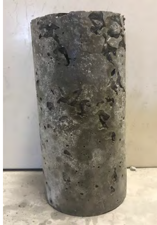
Figure 4.16 Example casted cylinder specimen with inadequate paste
