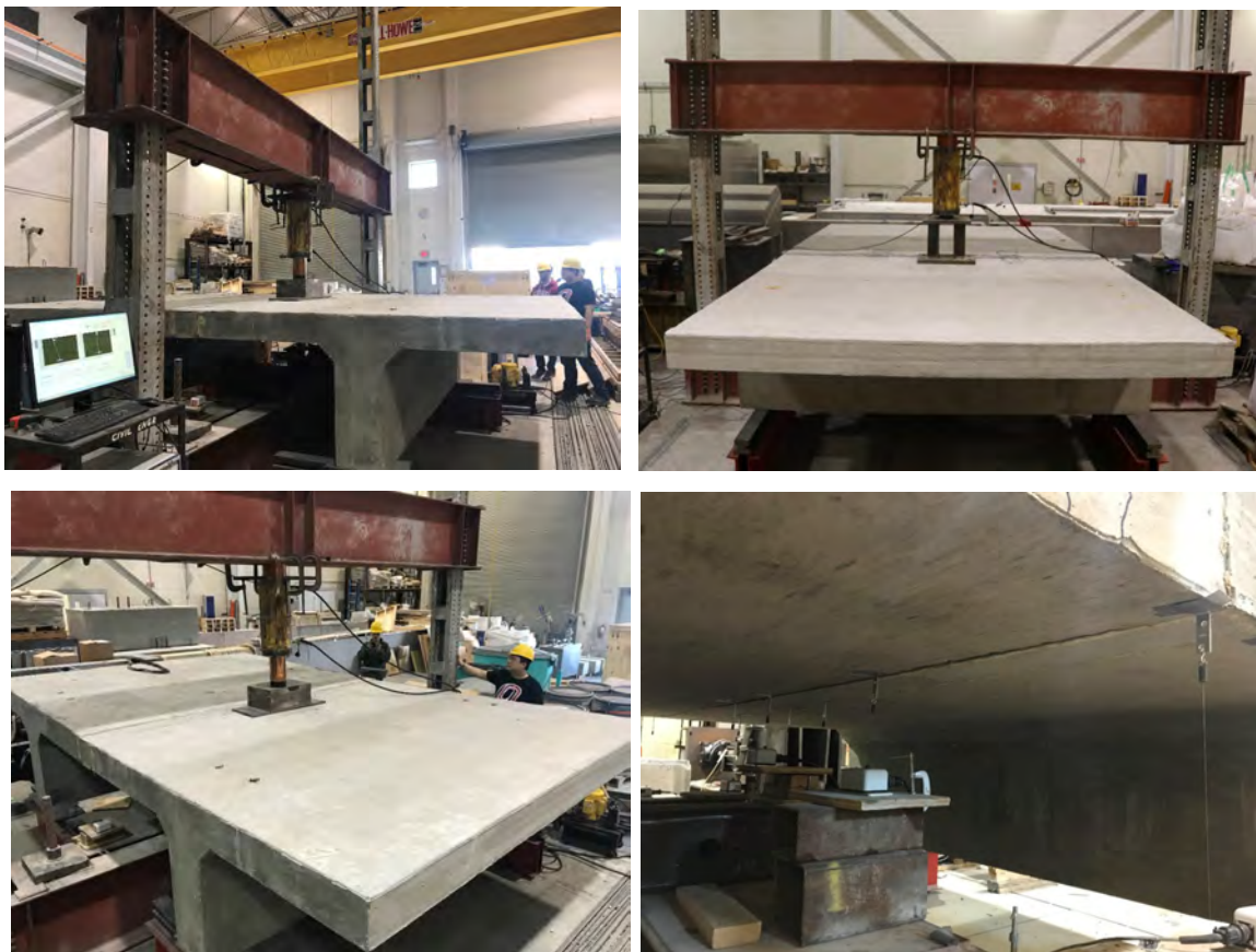
Figure 6.21 Full-scale slab connection specimen test setup
