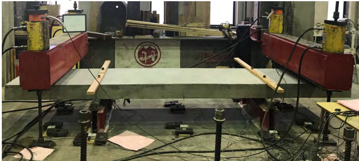
Figure 6.14 Slab specimen test set up
