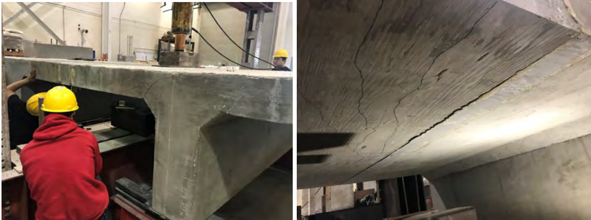
Figure 6.22 Crack mapping and failure of specimen F-R-SHPC
