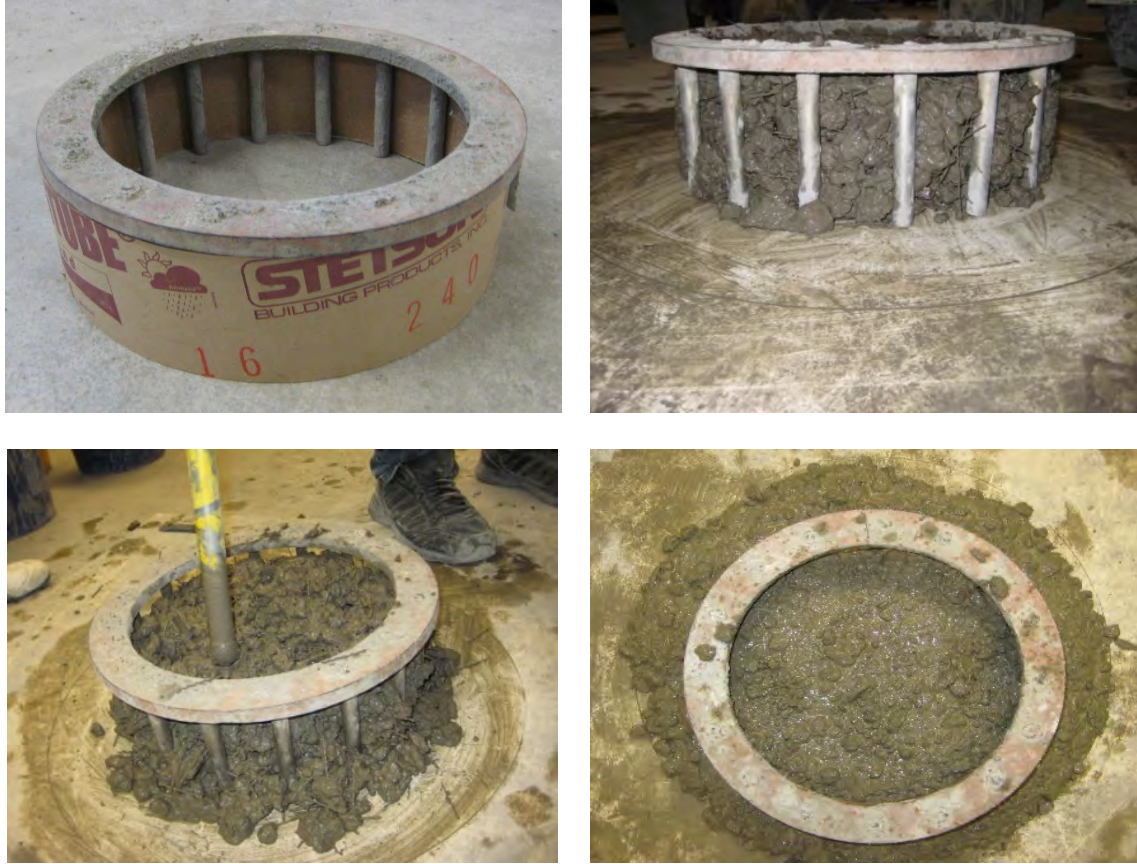
Figure 3.7 Vibrated J-Ring setup and test procedure
