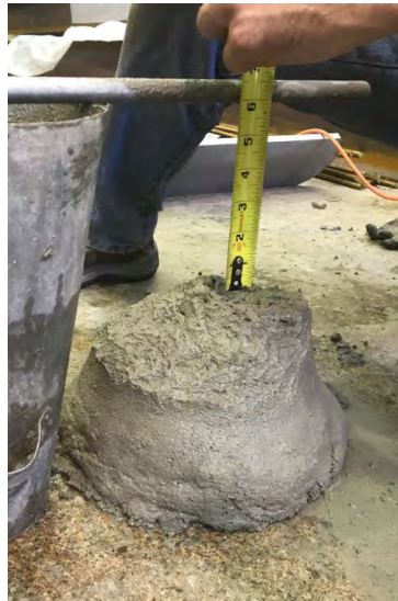
Figure 4.14 Comparison of Lincoln-Ref and FRC mix stability and appearance
