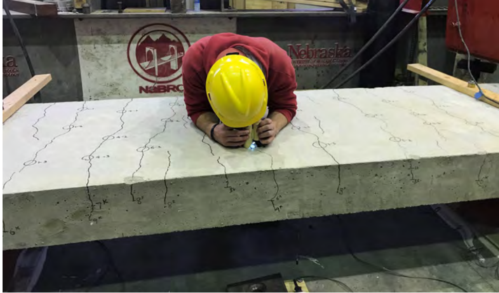
Figure 6.15 Crack width measuring during testing
