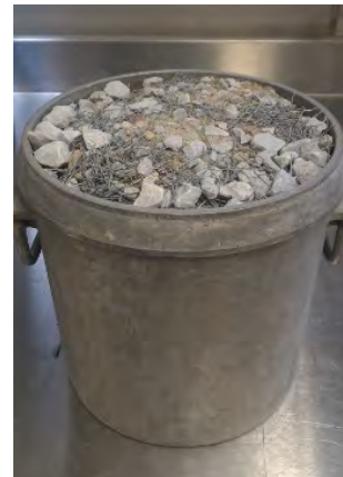
Leveled after consolidation
