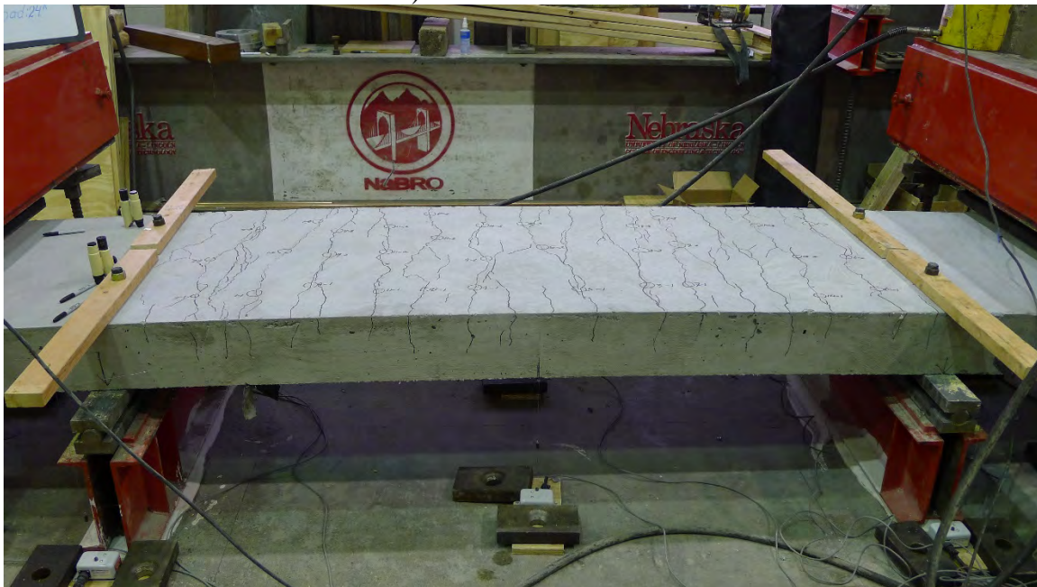
a) Fiber-reinforced concrete slab
