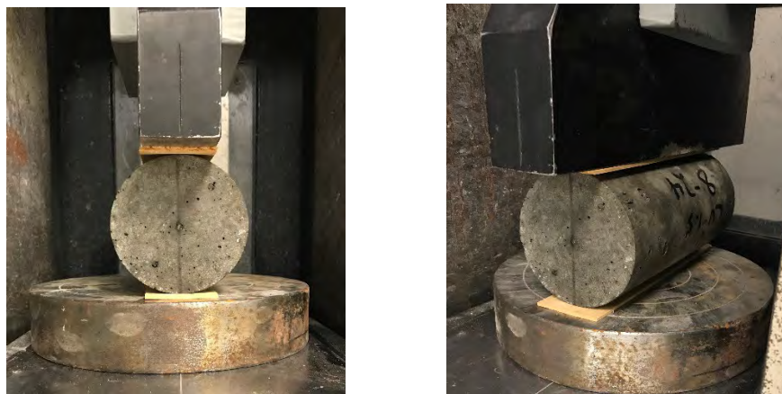
Figure 3.14 Test setup for splitting tensile strength
