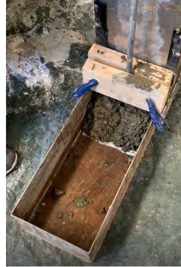
Figure 4.13 Comparison of LV-Ref and LV-FRC stability during vibrated L-Box test
