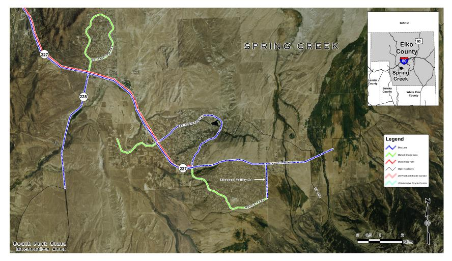
ELKO COUNTY SPRING CREEK Bicycles are to be accommodated on all roadways in Elko County. At a minimum, a paved shoulder with a minimum usable width of four feet should be included on all future roadway improvements with a speed limit over 25 miles per hour. Opportunities for additional bicycle facilities that are not identified in this bicycle plan may develop and should be pursued.
