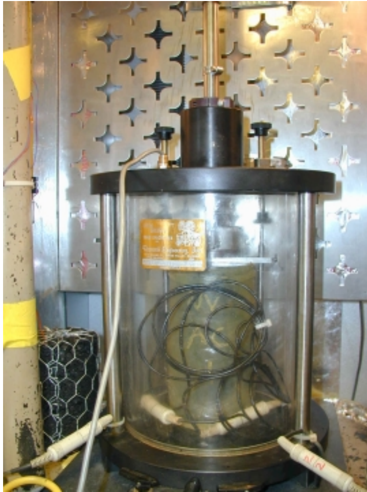
Figure 2 Repeated load triaxial test machine.
