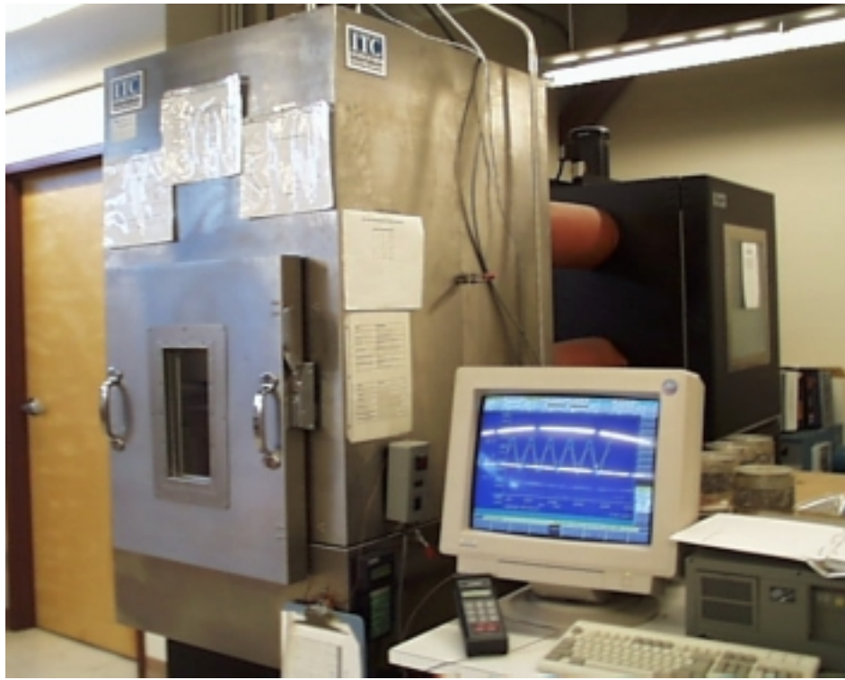
Figure 3 Superpave Shear Tester machine.
