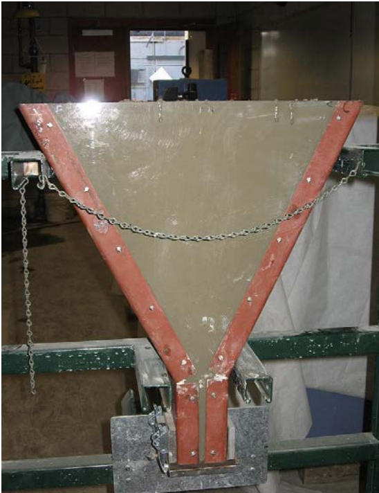
Figure 3.3: e) V-funnel (confined workability) and f) Column segregation (static segregation resistance) tests
