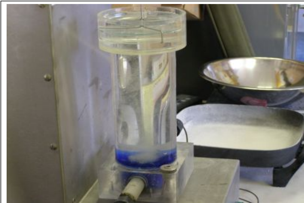
Figure 6.13: Air void analysis test in progress
