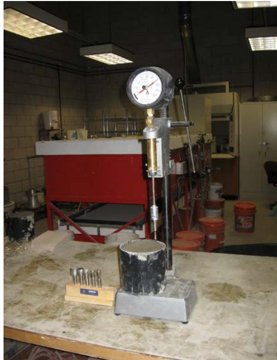
Figure 3.3: g) Adiabatic temperature and h) Setting time tests
