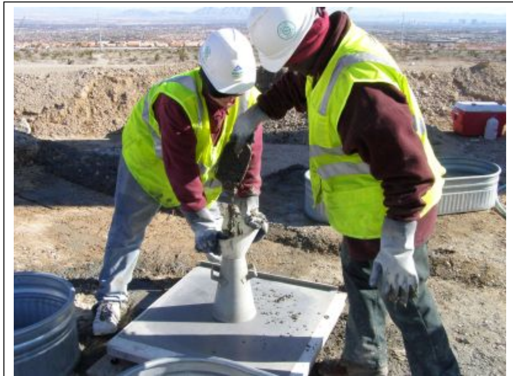
Figure 6.8a: Slump flow test
