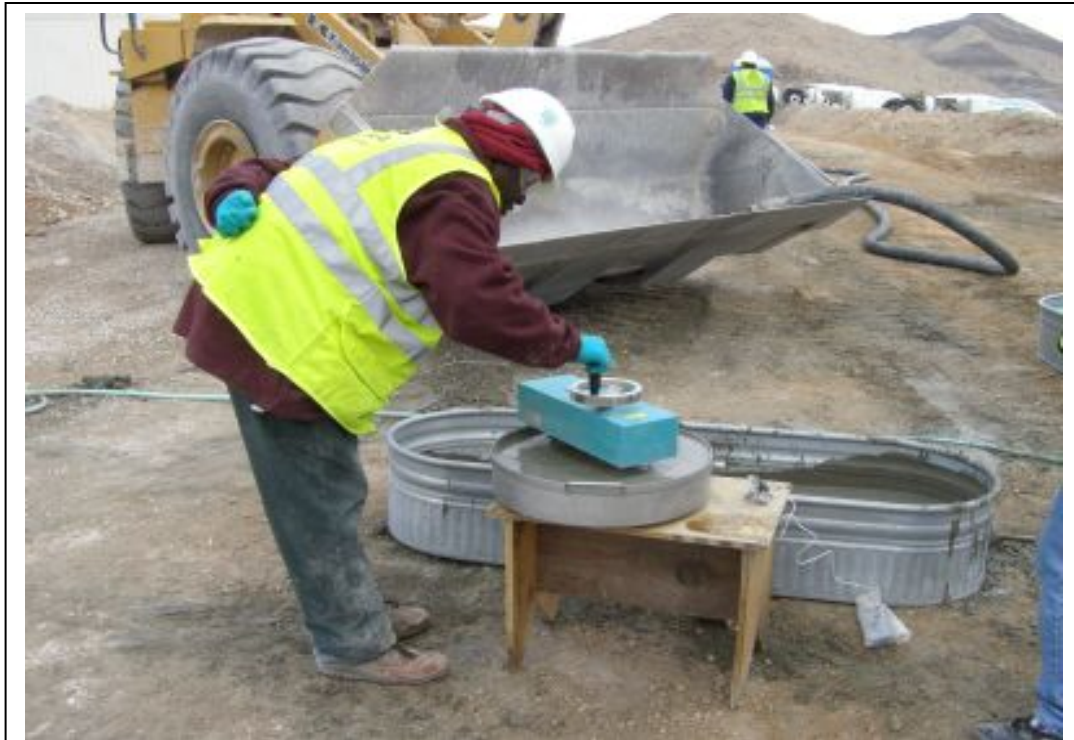
Figure 6.23: Rheology test measurement for pumped SCC
