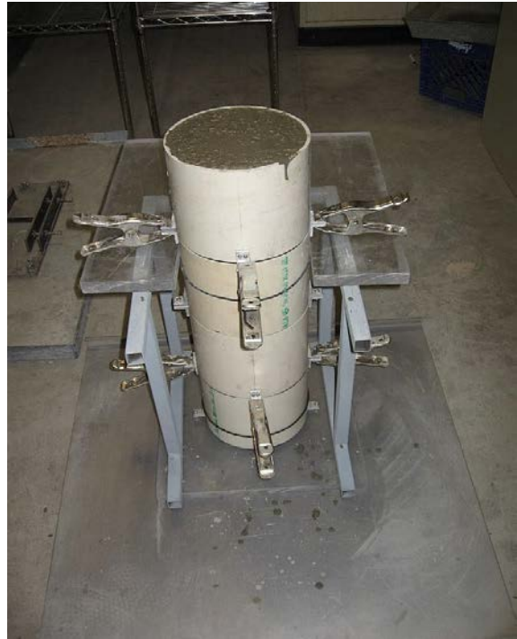
Figure 3.3: e) V-funnel (confined workability) and f) Column segregation (static segregation resistance) tests
