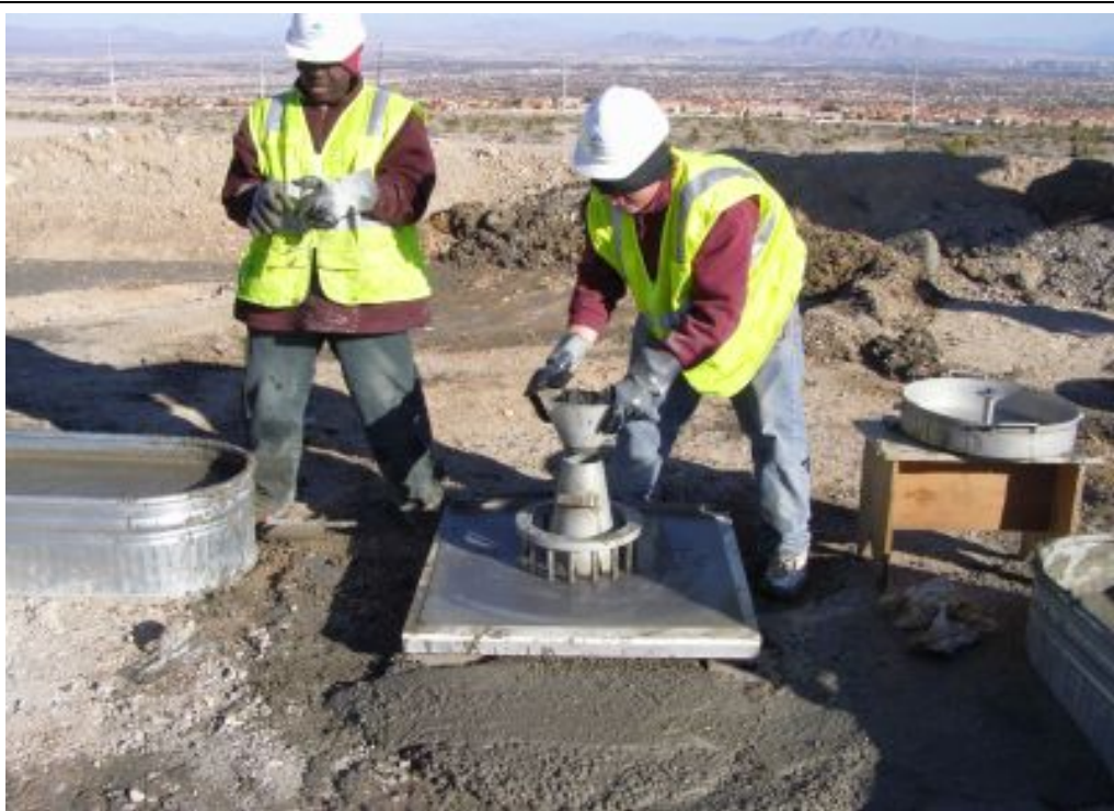
Figure 6.19: J-ring test for post-pumped SCC
