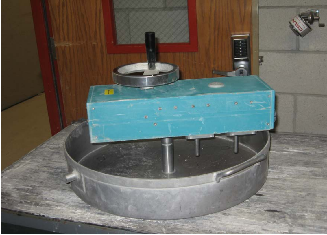
Figure 6.25: Two-point BT2 concrete rheometer
