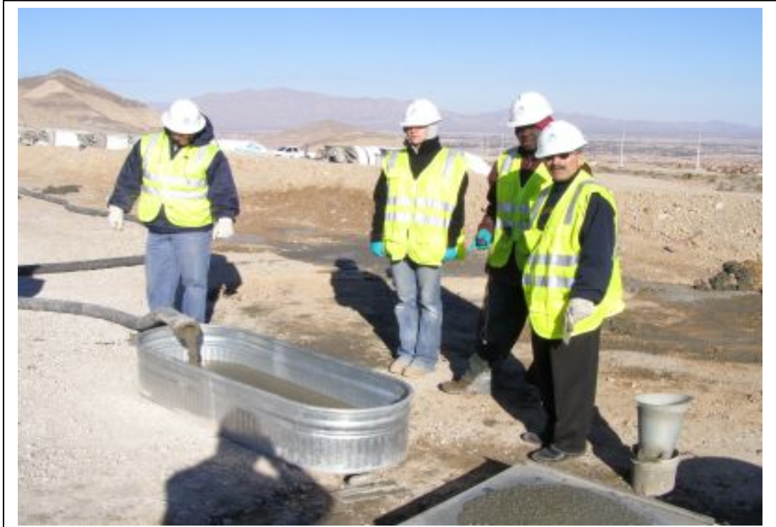
Figure 6.17: Pumping test - post-pumping SCC sample collection
