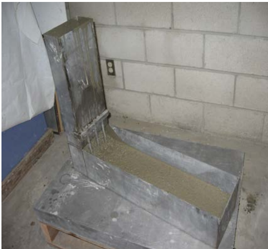
Figure 3.3: c) L-box (passing ability) and d) U-box (passing and filling ability) tests
