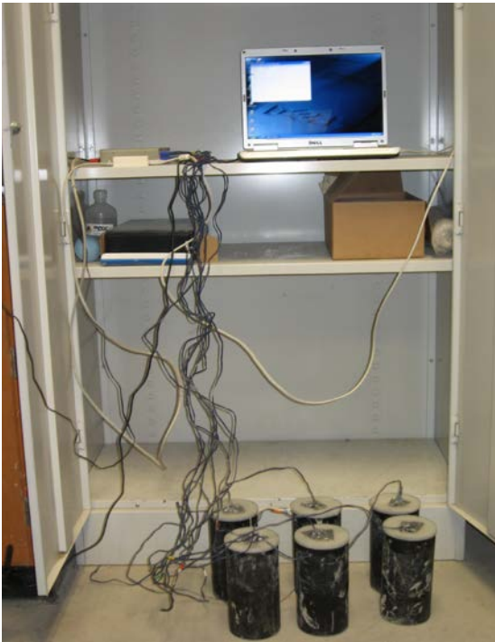
Figure 3.3: g) Adiabatic temperature and h) Setting time tests
