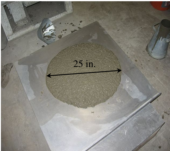
Figure 3.3: a) Slump flow (unconfined workability) and Visual stability index (VSI, dynamic segregation resistance), and b) J-ring (passing ability) tests
