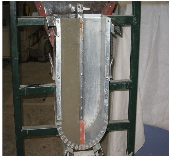
Figure 3.3: c) L-box (passing ability) and d) U-box (passing and filling ability) tests
