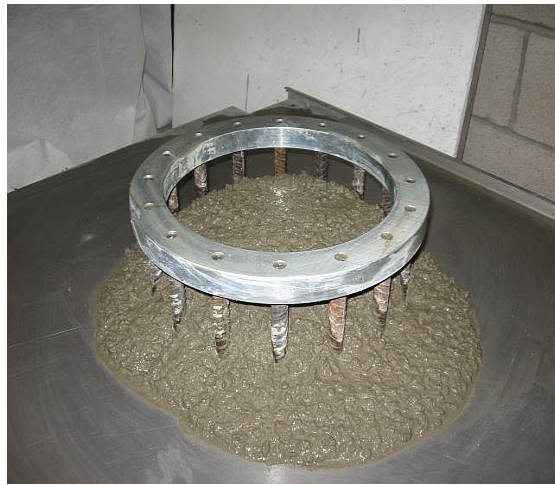
Figure 3.3: a) Slump flow (unconfined workability) and Visual stability index (VSI, dynamic segregation resistance), and b) J-ring (passing ability) tests
