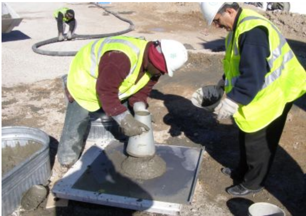
Figure 6.18b: Slump flow test for post-pumped SCC (continued)
