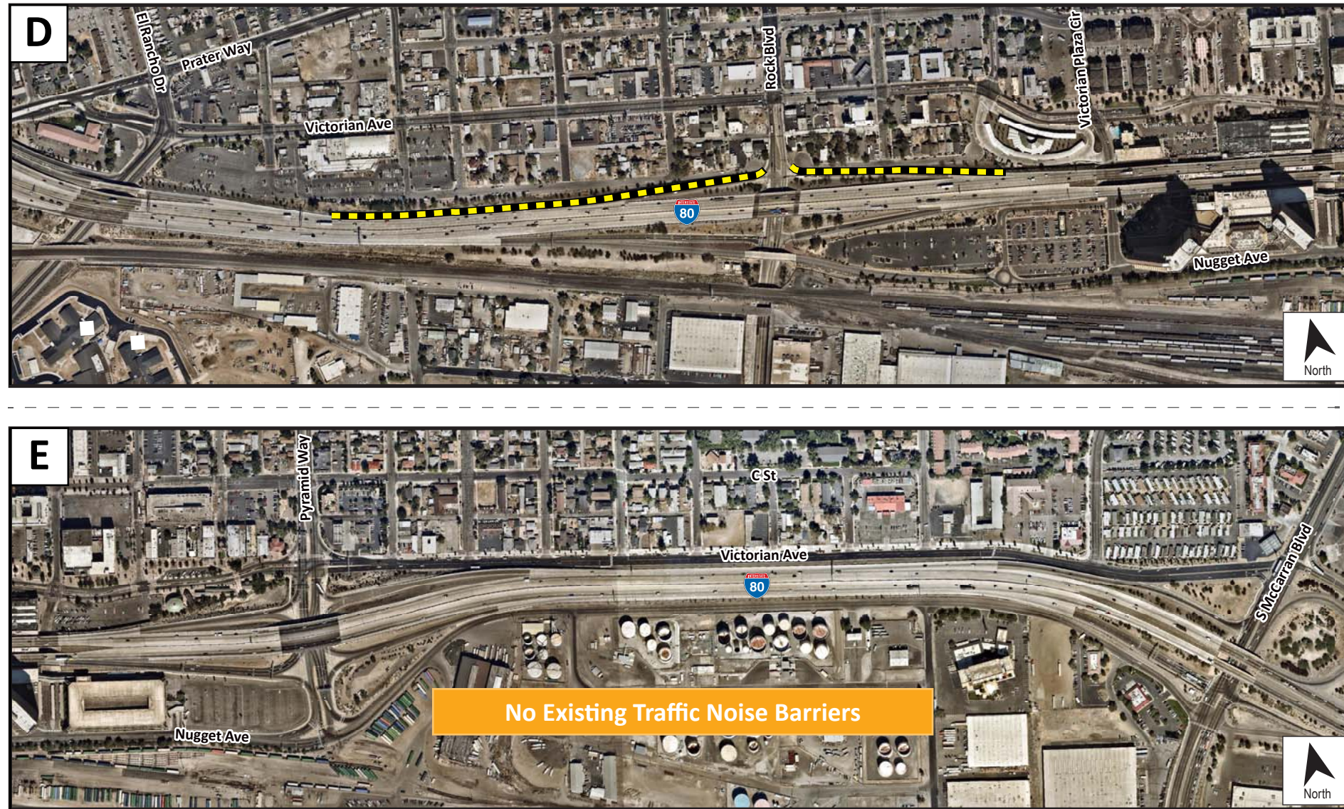
Figure 3.4-1B. Locations of Existing Traffic Noise Barriers (East-West)
