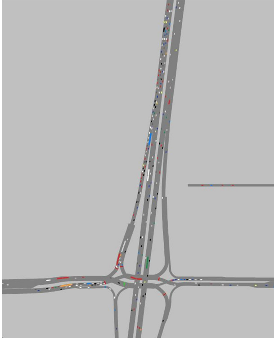
Figure 6: Moana Ln Off-Ramp Queue extending on to mainline during PM Peak Period
