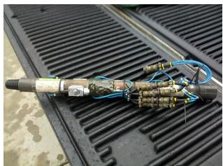
The SPT Analyzer is fully compliant with the minimum digital sampling frequency requirements of ASTM D4633-05 (50 kHz) and EN ISO 22476-3:2005 (100 kHz), as well as with the low pass filter, (cutoff frequency of 5000 Hz instead of 3000 Hz) requirements of ASTM D4633-05. All equipment and analysis also conform to ASTM D6066.
