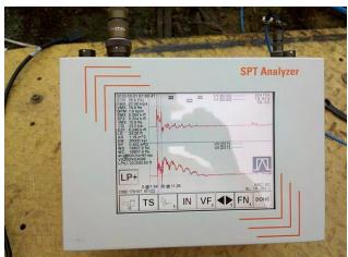
An SPT Analyzer from Pile Dynamics was used to record and process the data. The raw data was stored directly in the SPT Analyzer computer with subsequent analysis in the office with PDA-W and PDIPlot software. The measurements and analysis were conducted in general accordance with ASTM D4945 and ASTM D6066 test standards.
