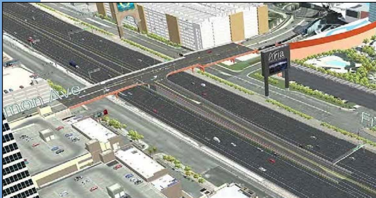
View of the Harmon HOV ramps connecting from I-15 to the south side of the existing Harmon Avenue overpass.
