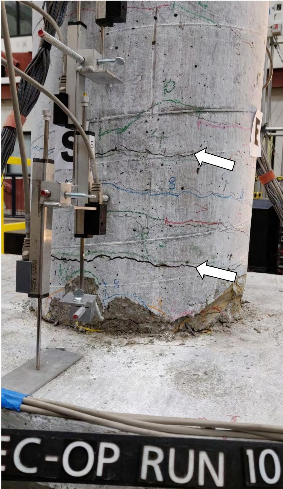
Figure 5.13 Flexural cracks widening after run 10
