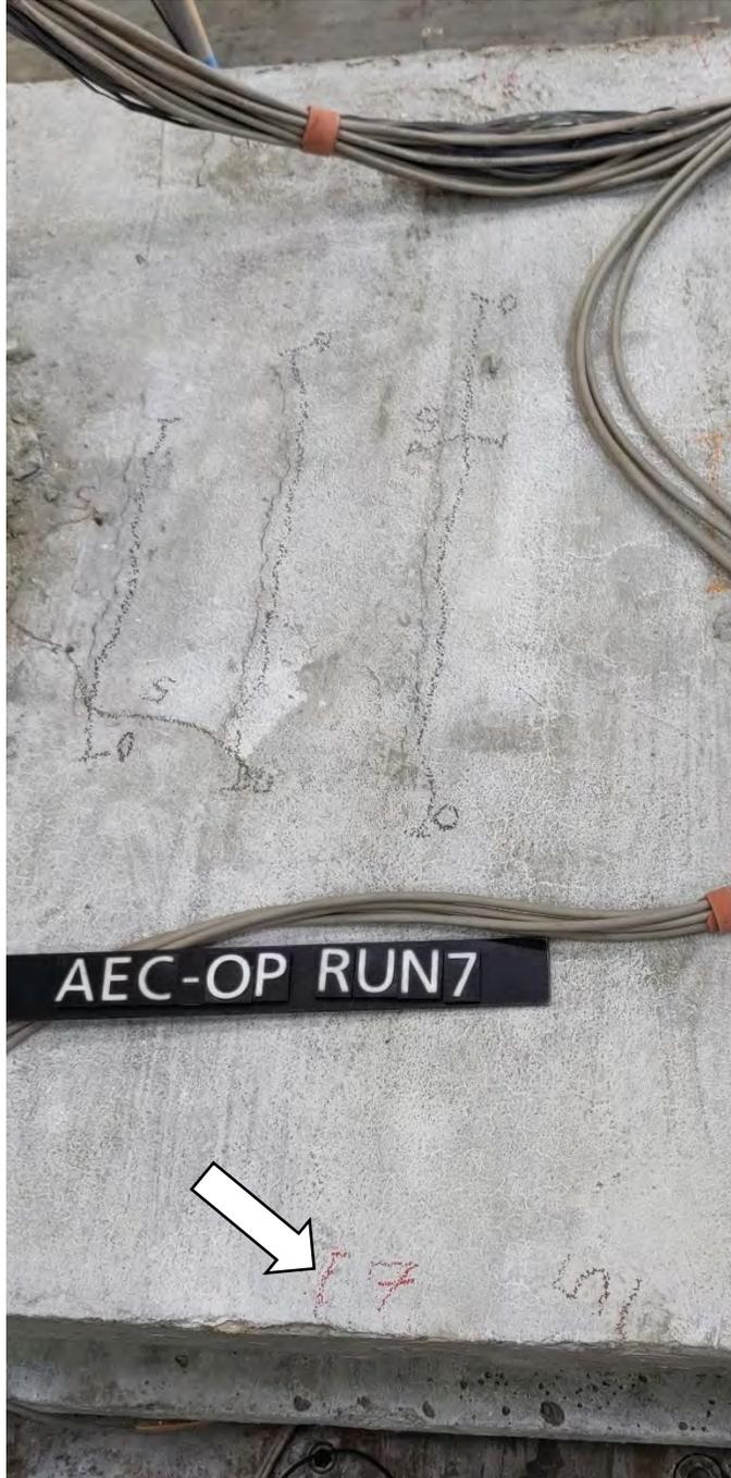
Figure 5.9 Torsion crack in cap beam flange after run 7
