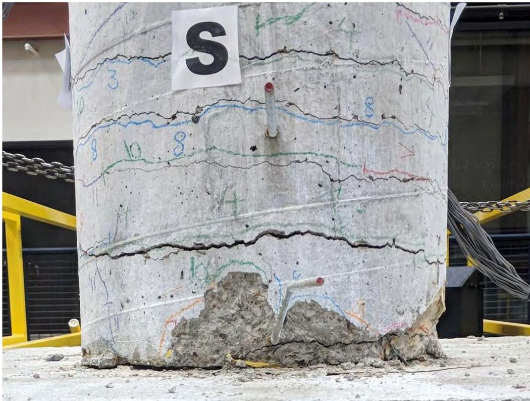
Figure 5.15 Concrete spalling on column south side after run 11 (final run)
