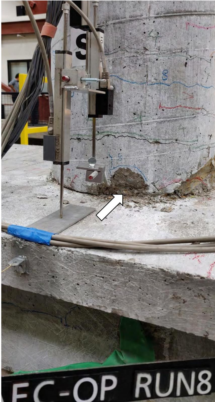
Figure 5.8 Concrete spalling on column south side after run 8
