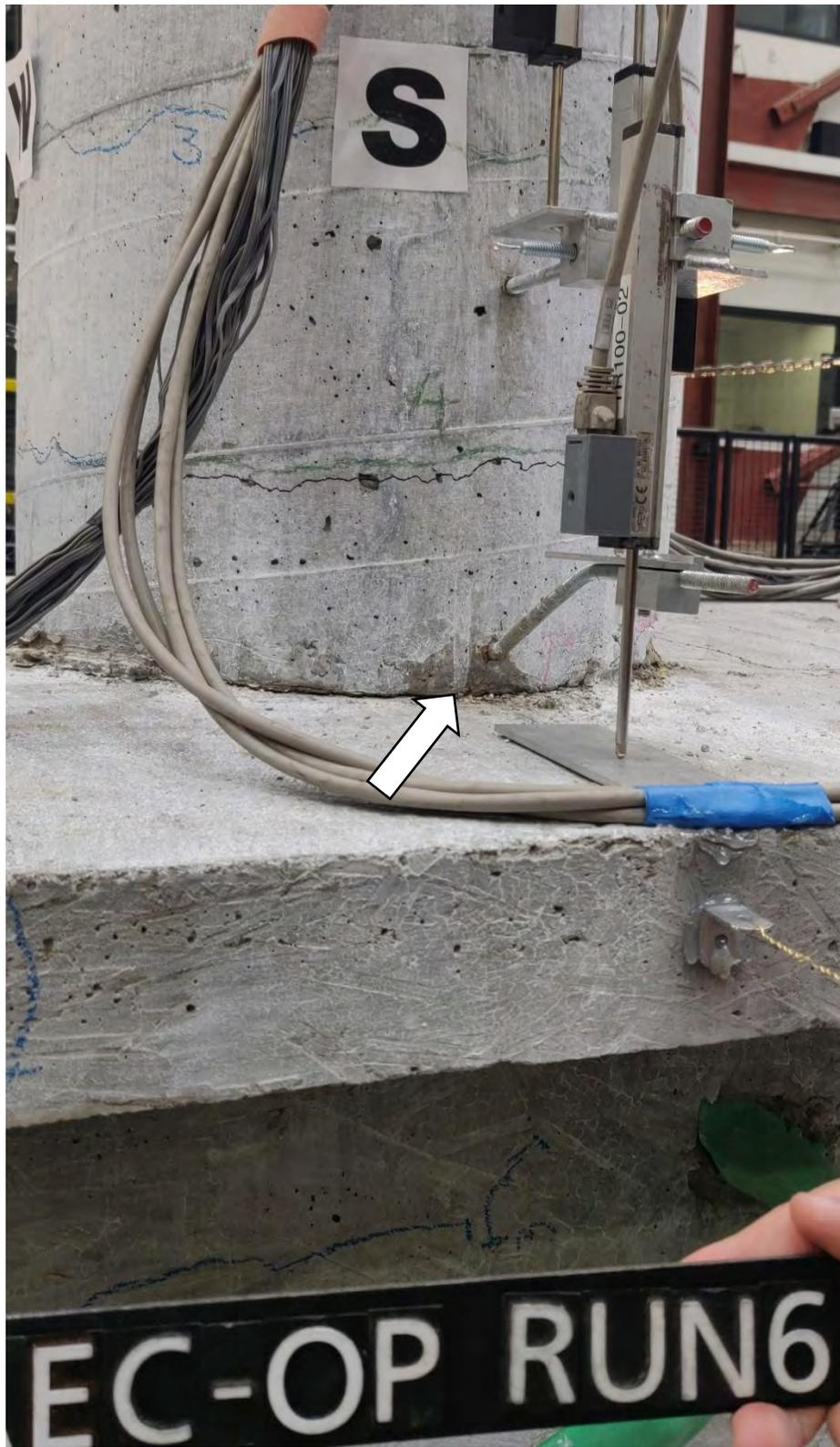
Figure 5.7 Concrete spalling on column south side after run 6
