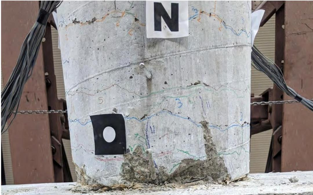
Figure 5.14 Concrete spalling on column north side after run 11 (final run)
