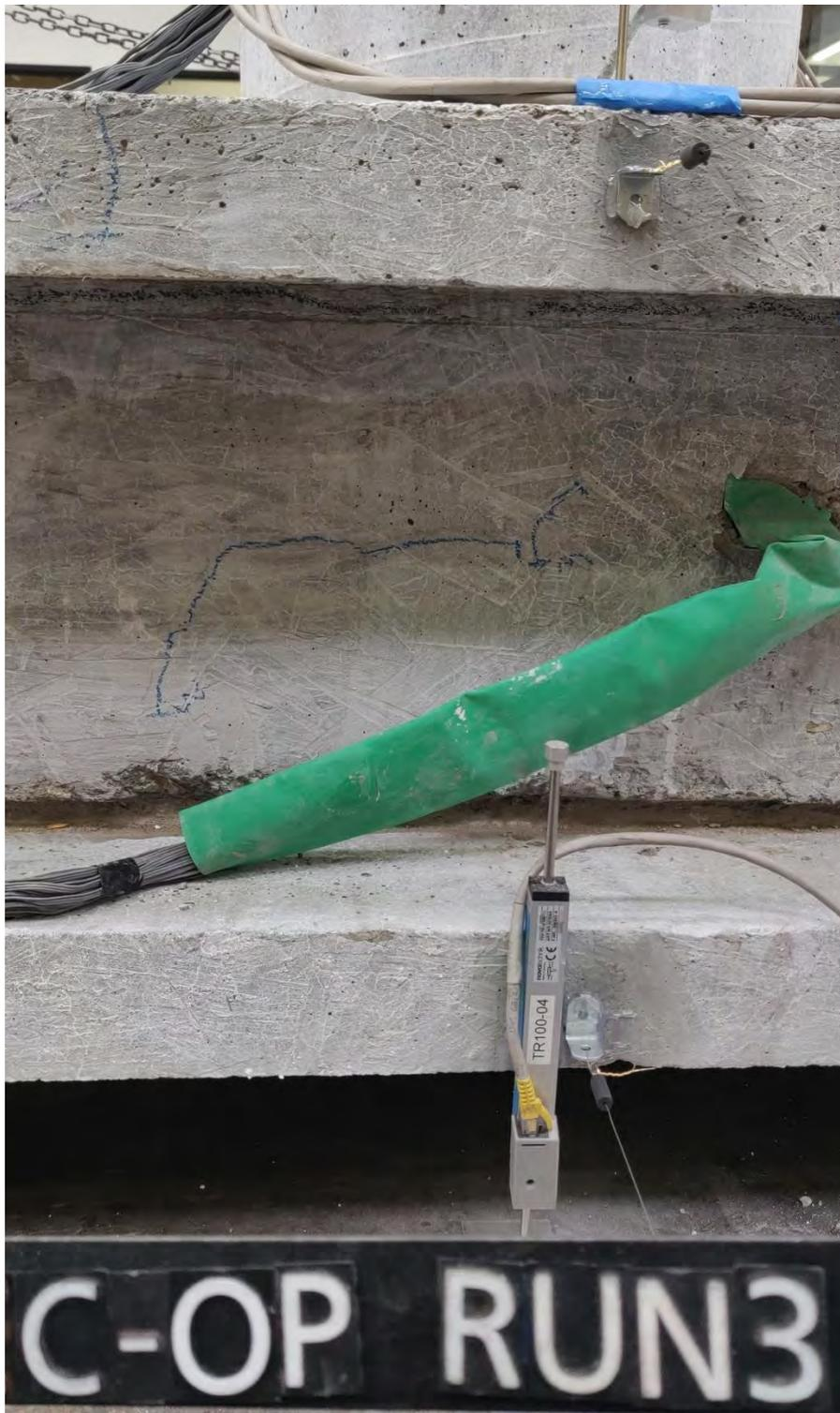
Figure 5.4 Shear and torsion cracks on cap beam south side after run 3
