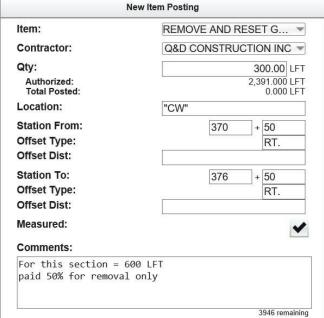
Figure 17-8: DWR Item Posting – Guardrail Remove and Reset LFT
