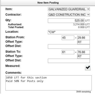
Figure 17-6: DWR Item Posting - Guardrail LFT
