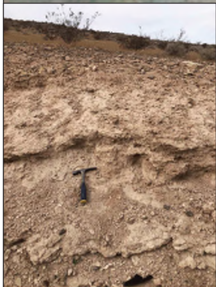
Calcrete , whiteish pink, moderately cemented, dry, nonplastic, fine to coarse sand, fine subangular gravel
