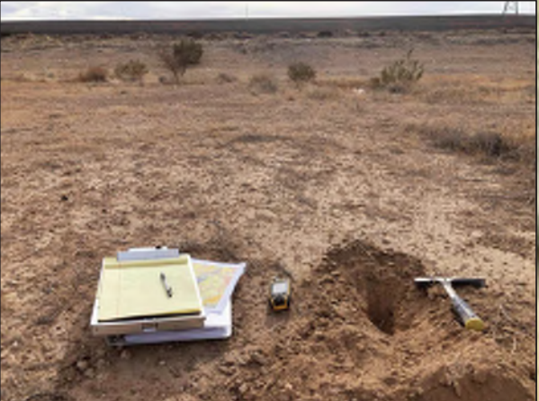
Clayey Sand with Gravel (SC), reddish brown, dry, low plasticity, fine sand, fine and coarse subrounded to subangular gravel
