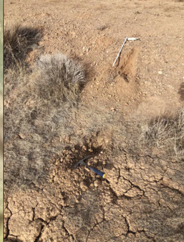
Clayey Gravel with Sand (GC), light brown, dry, low plasticity, fine sand, trace fine gravel, desiccation cracking and animal burrowing disturbances
