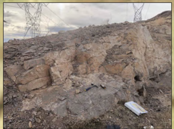
Bird Springs Formation: Quartzite, grey-white, massive, jointed and fractured, R4, with calcite infill (contact exposed in cut face)
