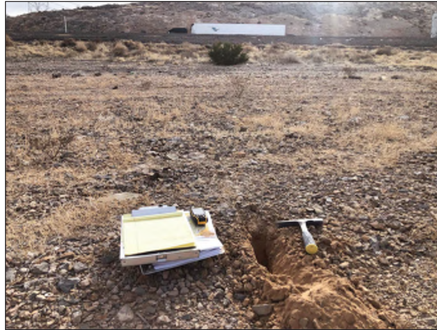
Silty Gravel with Sand (GM) , reddish brown, dry, nonplastic, fine sand, fine and coarse subangular to angular gravel, with cobbles
