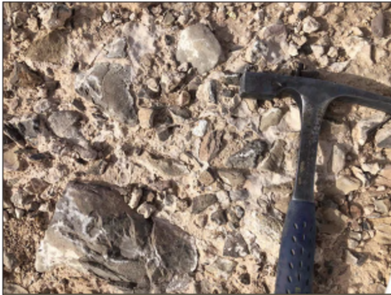
Calcrete , tannish white, moderately to strongly cemented subangular to angular gravels and cobbles, fine and coarse gravel
