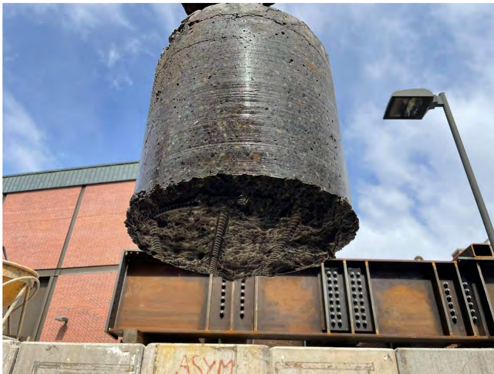
Figure 2.8 Close-up view of the extracted portion of the column (embedded in joint)
