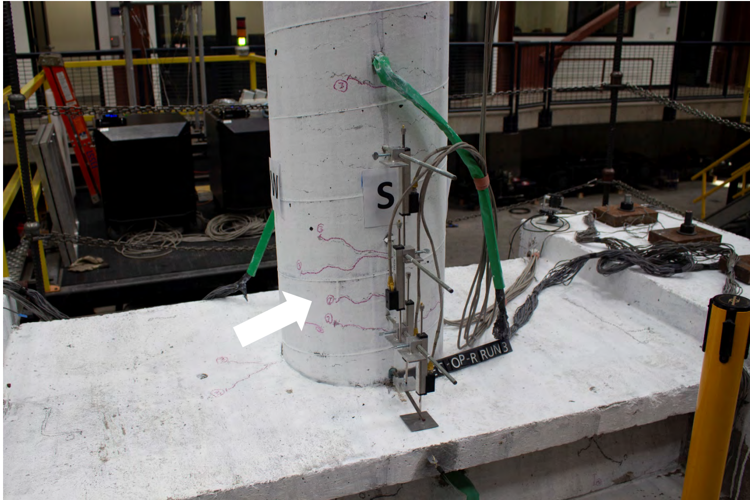
Figure 3.2 Additional flexural cracks (run #3)
