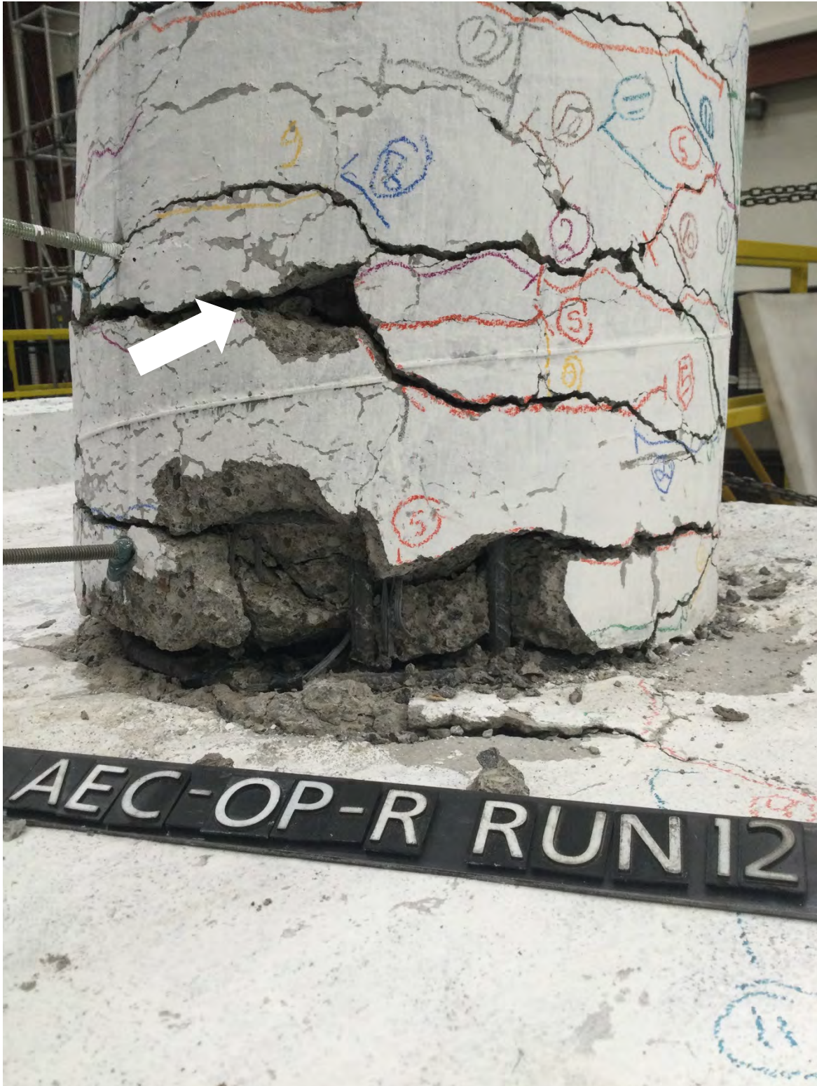
Figure 3.17 Spalling and widening of flexural cracks on the south side (run #12)
