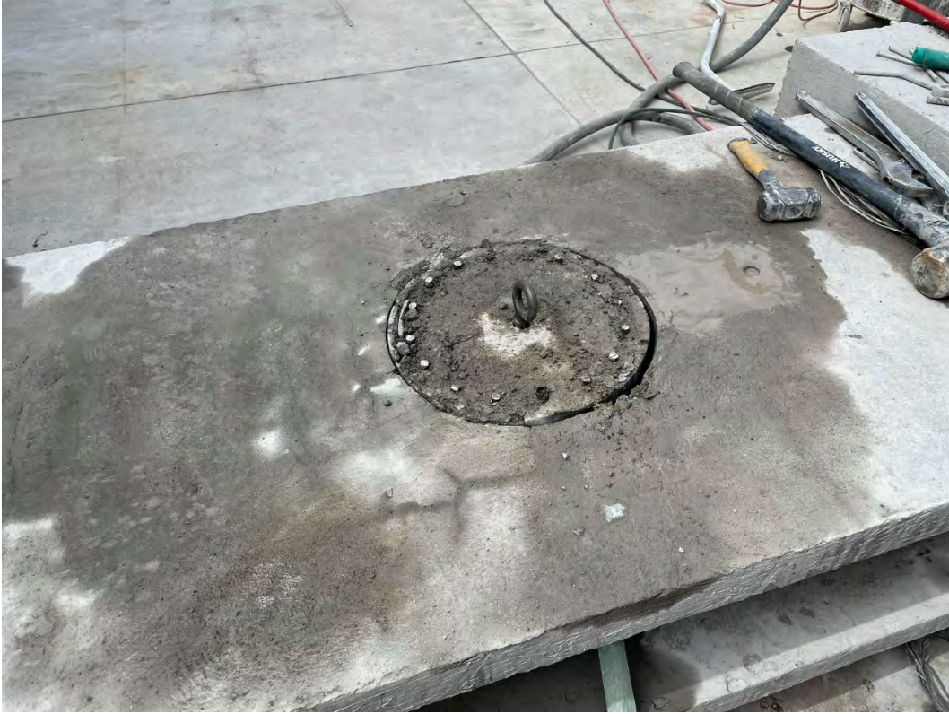
Figure 2.5 Cap beam specimen after cutting
